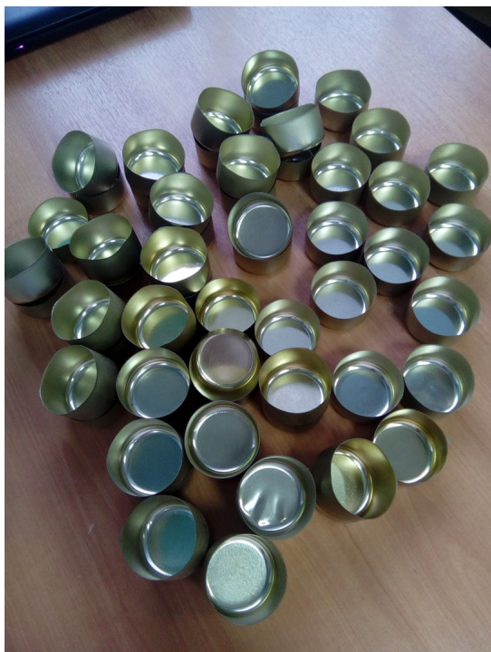
Figure 3. Cans Coated with Coating Composition from Synthesized Polyester Containing Fragments of Sunflower Oil Fatty Acid: View after Sterilization in Drinking Water
