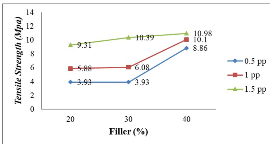
Fig.1: Relation between Tensile Strength of Bio Composite with different ratio of Filler and Matrix.
