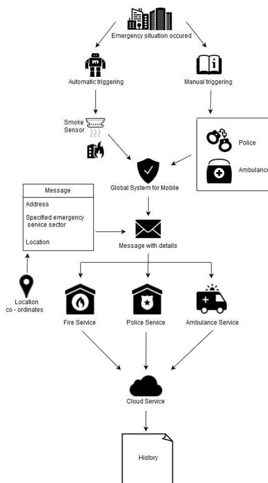
Figure 1: System architecture
