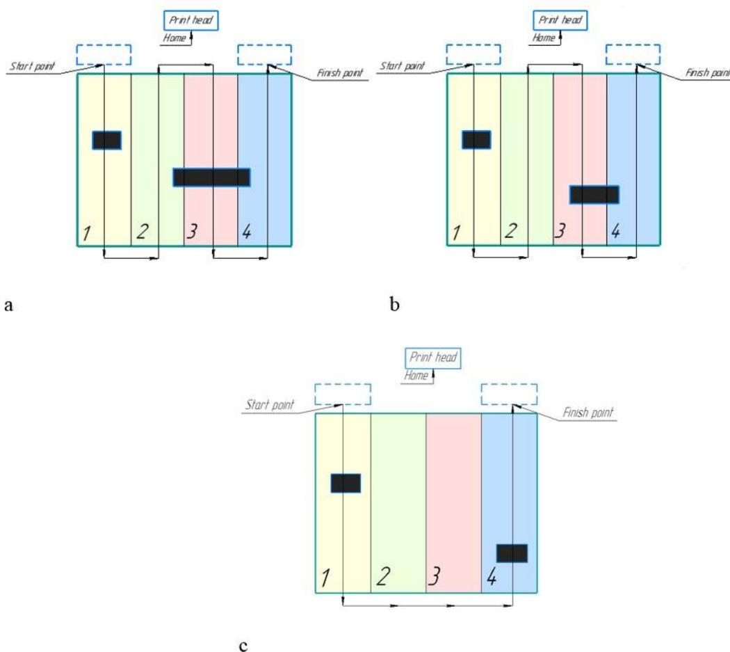
**Fig 3:** Movement of the print head without optimisation: a – details are situated in all sectors; b – details are situated in 1, 3, and 4 sectors; c – details are situated in 1 and 4 sectors.
