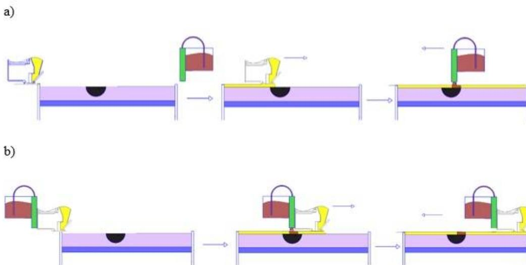
**Fig2:** a – separated structure of the entire device; b – combination of the device for application of the sand and the unit of print heads
