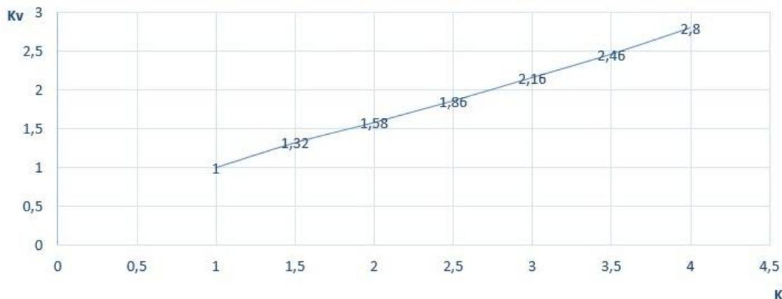
**Fig. 8:** Chart of dependencies of the coefficient of improvement of the rate of printing  $K_v$  from the coefficient of increase in dimensions of the drops  $K$
