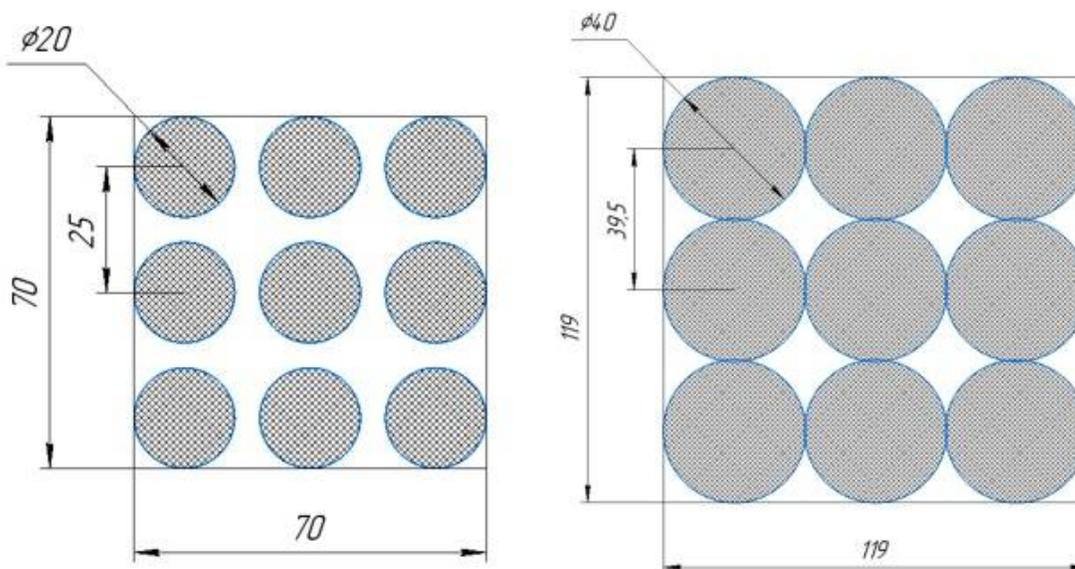
**Fig 6:** Changing step of ejection of the drops in the case of increase in dimensions of the drops
