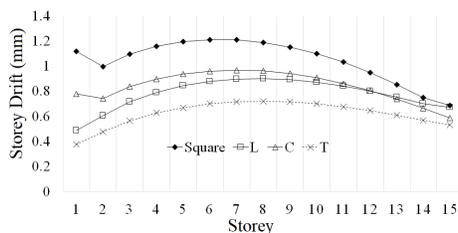
**Fig 5(b):** Storey drift along y-direction due to  $E_y$
