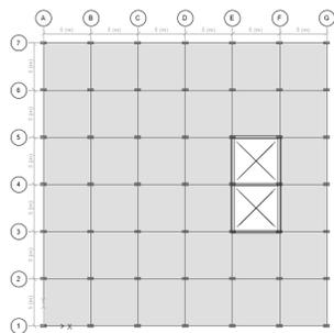
**Fig 1:** Regular Symmetrical Square Shape Building Plan
