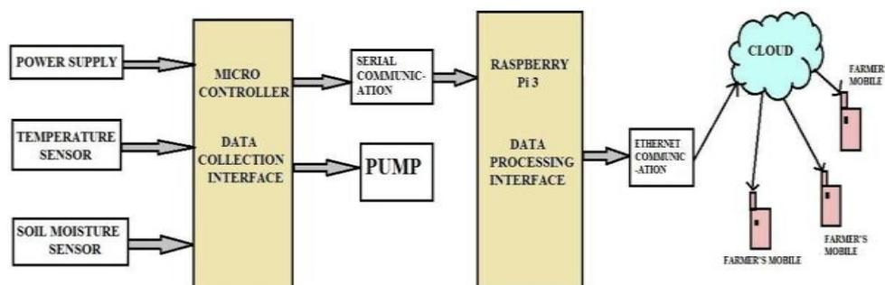
Figure 1: IOT based automated irrigation system
