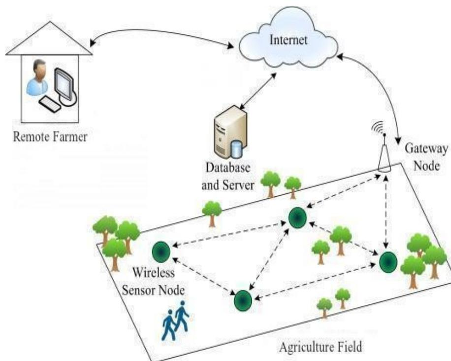
Figure 4: Architecture diagram
