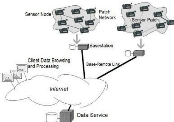
Figure 2: Architecture of Bottom System
