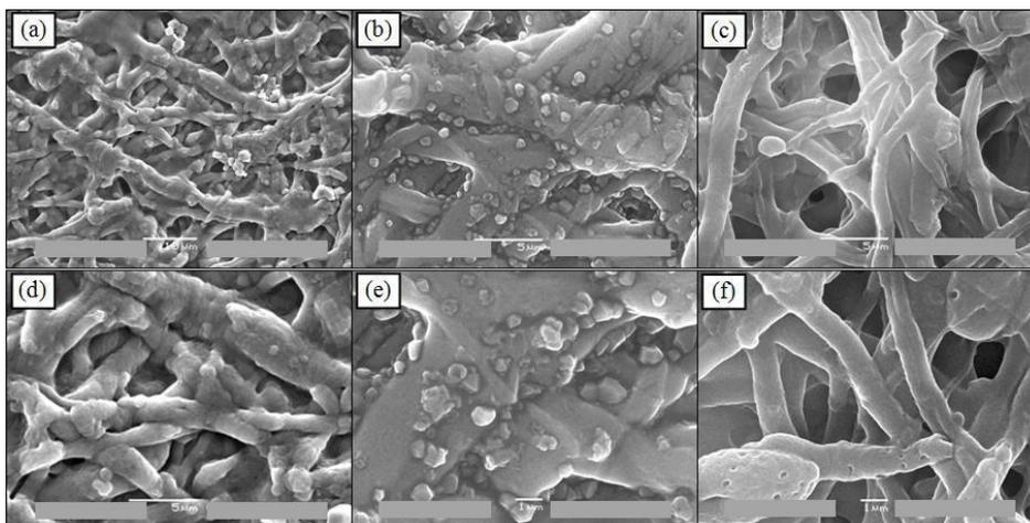
**Fig 2:** SEM images of scaffold after incubation process in modified SBF Kokubo solution for: (a) 6; (b) 9; and (c) 12 days.
