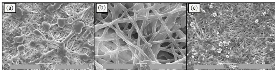
**Fig 1:**Microstructure of eggshell membrane: (a) before immersing in NaOH solution; (b) Fig. 1a with higher magnification; (c) after immersing in NaOH solution.
