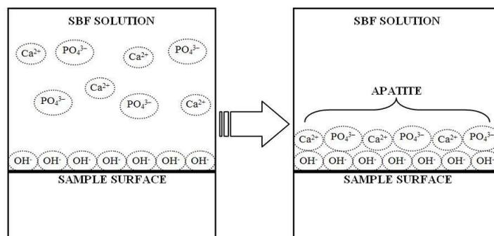
**Fig 4:** Illustration of apatite formation on membrane surface.
