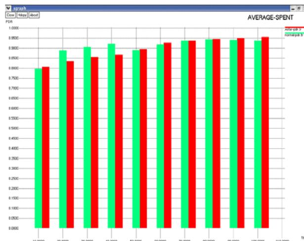
Fig. 9: Packet delivery ratio for AODV and A-STAR Conclusion
