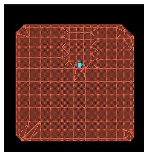
Figure 4: Microstrip patch Antenna – ADS Layout
