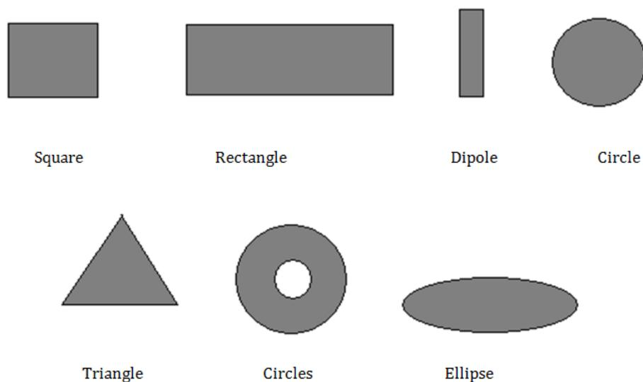
Figure 2: Different shapes of Microstrip patch Antenna
