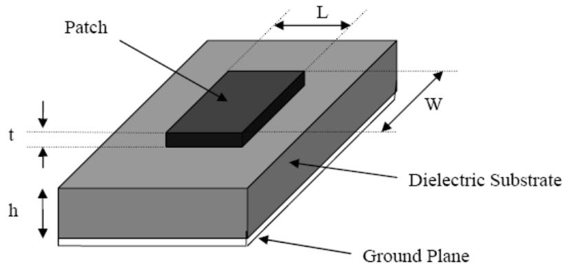
Figure 1: Structure of a Microstrip Patch Antenna
