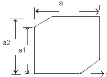
Figure 3: Microstrip patch antenna with truncated corners
