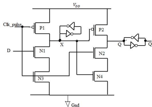
Fig. 1: Double edge triggered explicit-pulsed flipflop (ep-DCO flipflop)
