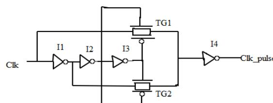
Fig. 2: Clock pulse generator used for Double edge triggering
