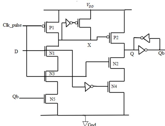
Fig. 3: Conditional Discharge Double-edge triggered Flipflop
