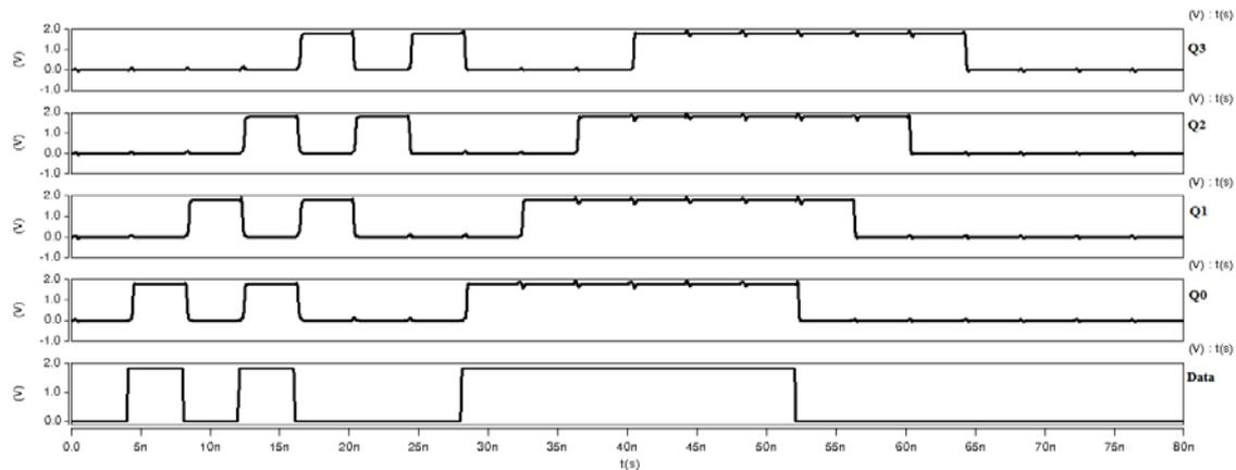
Fig. 10: 4 bit shift register output of MTCMOS CDFD flip flop
