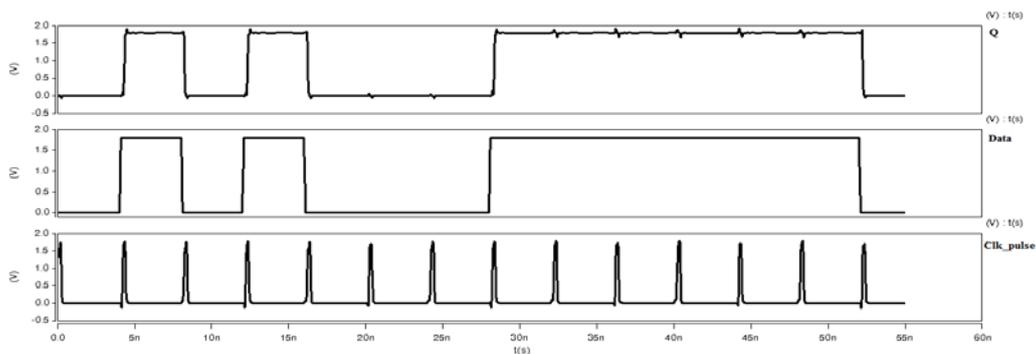
Fig. 9: Hspice simulated output wave form of MTCMOS CDFF flip flop
