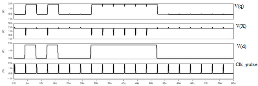
Fig. 7: Hspice simulated output wave form of EP-DCO flip flop
