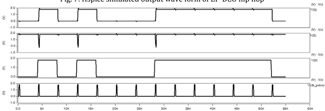
Fig. 8: Hspice simulated output wave form of CDFF flip flop
