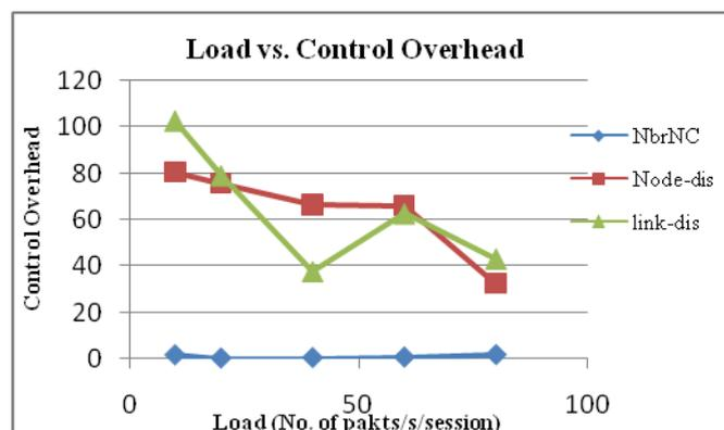
Fig. 10: Variation of Control Overhead with network load
