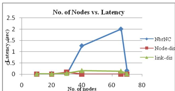
Fig. 8: Variation of Latency with network size
