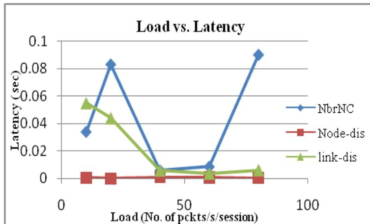
Fig. 11: Variation of Latency with network load
