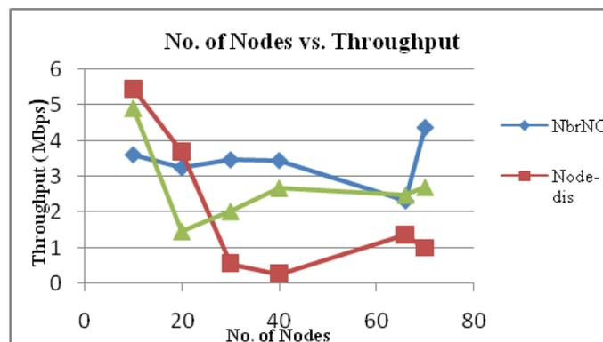
Fig. 6: Variation of throughput with network size
