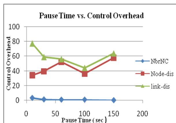
Fig. 13: Variation of Control Overhead with Pause Time
