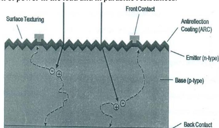
Figure 1: Basic structure of simple solar cell
