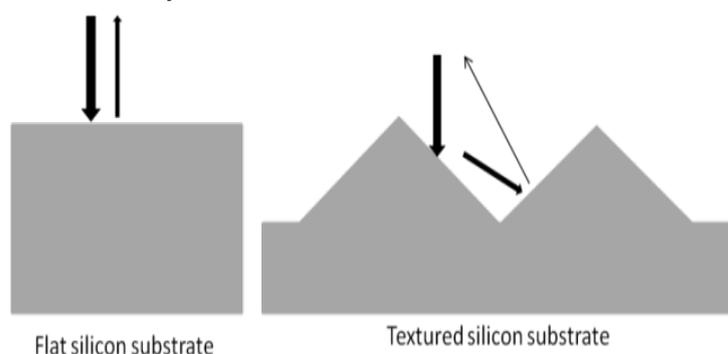
Figure2: Reflection of light from flat and textured surface
