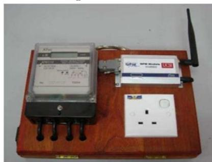
Figure 3: GSM PowerMeter
