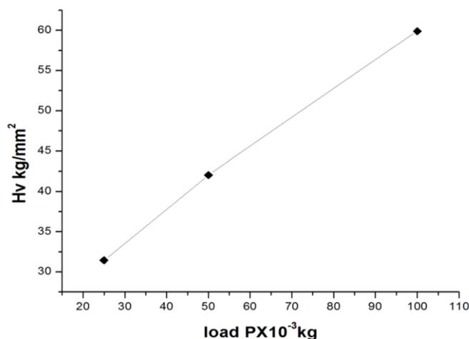
Figure 6: Variation of hardness with load for ZSH crystal
