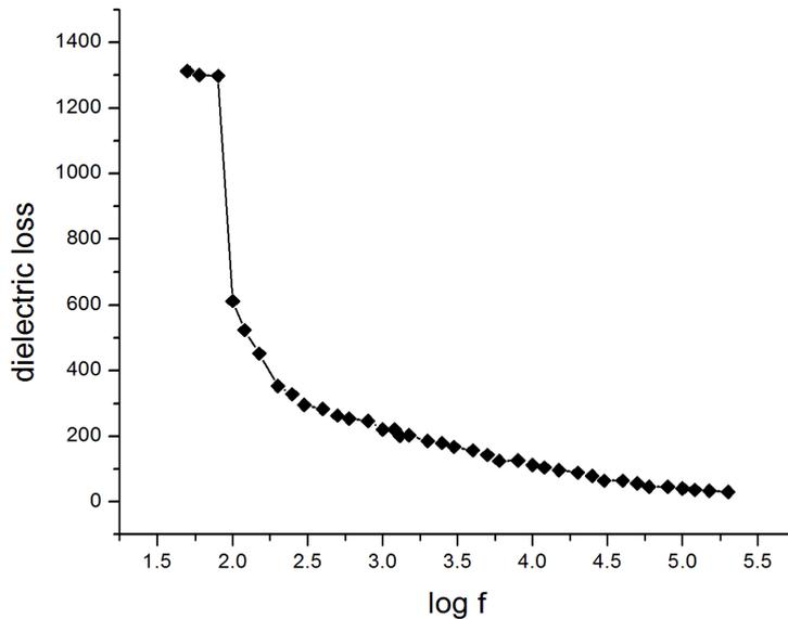
Figure 5: Variation of dielectric loss with frequency at room temperature
