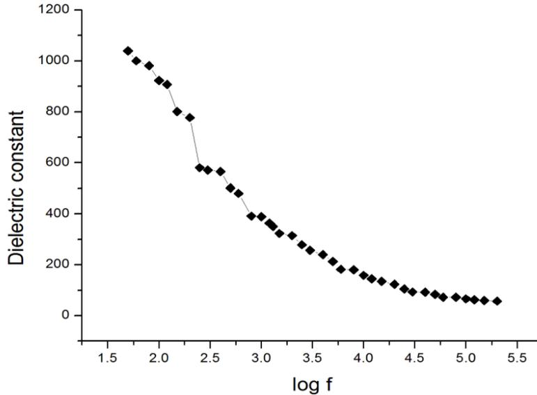
Figure 4: Variation of dielectric constant with frequency at room temperature
