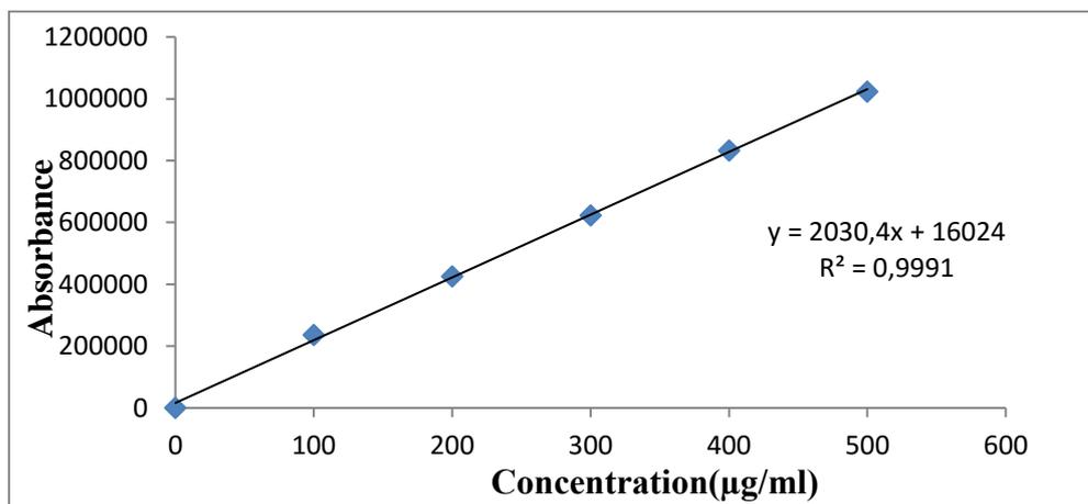
Figure 3: Calibration plot of Losartan
