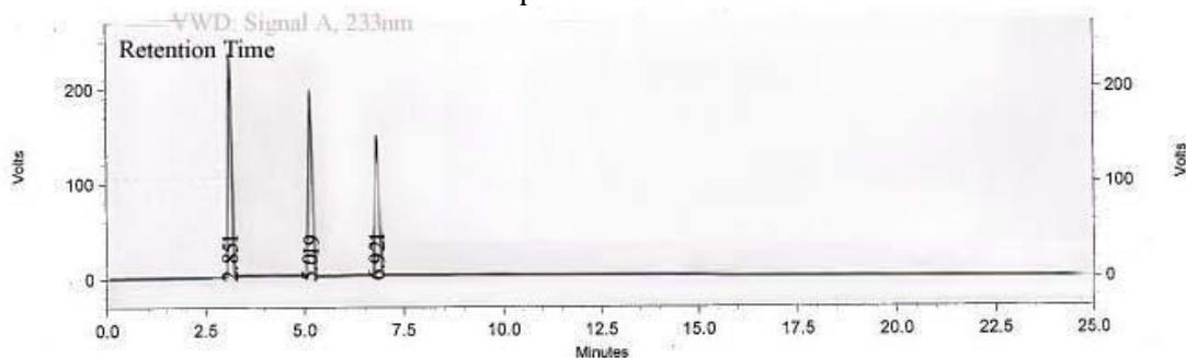
**Figure 6:** A typical chromatogram for assay of marketed formulation containing 10 $\mu$ g/ml of Losartan, 1 $\mu$ g/ml of Ramipril and 2.5 $\mu$ g/ml Hydrochlorothiazide
