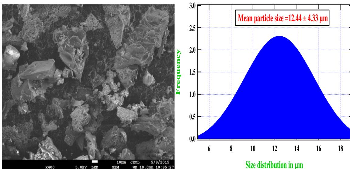
**Figure 4.** SEM image and particle size distribution (Gaussian blue) of particulate emissions of cashew nuts at 700 °C
