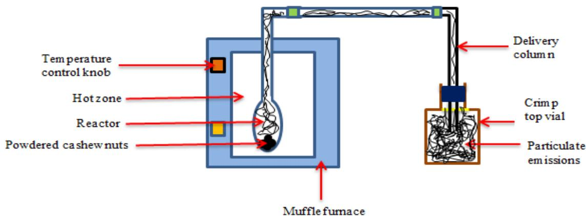
**Figure 1.** The reactor assembly and the gas-phase trapping apparatus for particulate emissions
