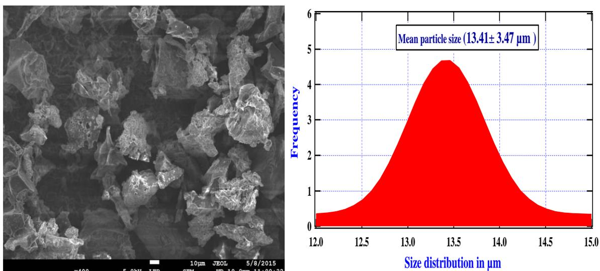
**Figure 3.** SEM image and particle size distribution (Gaussian red) of particulate emissions of cashew nuts at 500 °C
