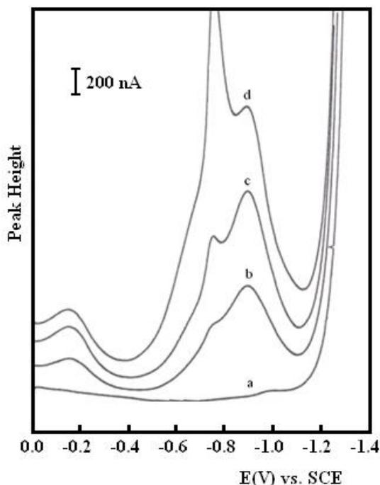
**Figure 2.** Determination of  $1 \times 10^{-5}$  M As(V) in the presence of  $5 \times 10^{-5}$  M Ti(III), **(a)** 10 mL 1M HAc/Ac (pH=2), **(b)** a + 0.1 mL sample, **(c)** b + 0.1 mL sample, **(d)** c + 0.1 mL  $1 \times 10^{-3}$  M As(III). (Sample:  $1 \times 10^{-3}$  M As(V),  $5 \times 10^{-3}$  M Ti(III), 1 M HCl)
