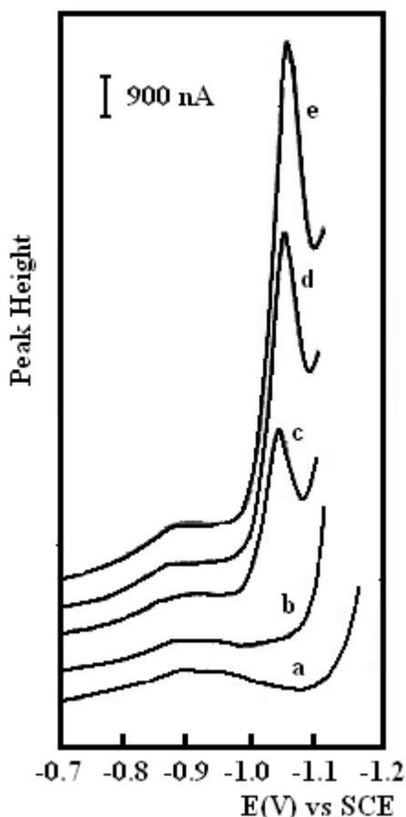
**Figure 3.** Determination of As(III) in beer sample using the catalytic hydrogen peak, **(a)** 10 mL 0.2 M HAc electrolyte (pH=3.2), **(b)** a + 0.05 mL  $2 \times 10^{-3}$  M Mo(VI), **(c)** b + 0.2 mL digested and reduced beer sample, **(d)** c + 0.1 mL  $1 \times 10^{-5}$  M As(III), **(e)** d + 0.1 mL  $1 \times 10^{-5}$  M As(III)
