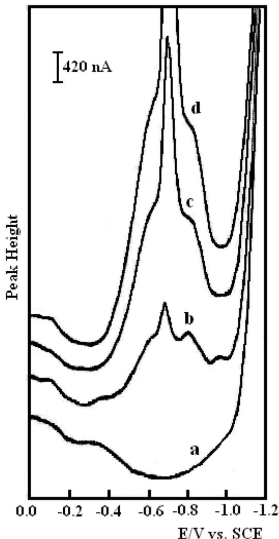
**Figure 1.** DP Polarographic behavior of As(III) in 0.1M HCl. **(a)** 10 mL 0.1 M HCl, **(b)** a + 0.1 mL  $1.0 \times 10^{-3}$  M As(III), **(c)** b + 0.1 mL  $1.0 \times 10^{-3}$  M As(III), **(d)** c + 0.1 mL  $1.0 \times 10^{-3}$  M As(III)
