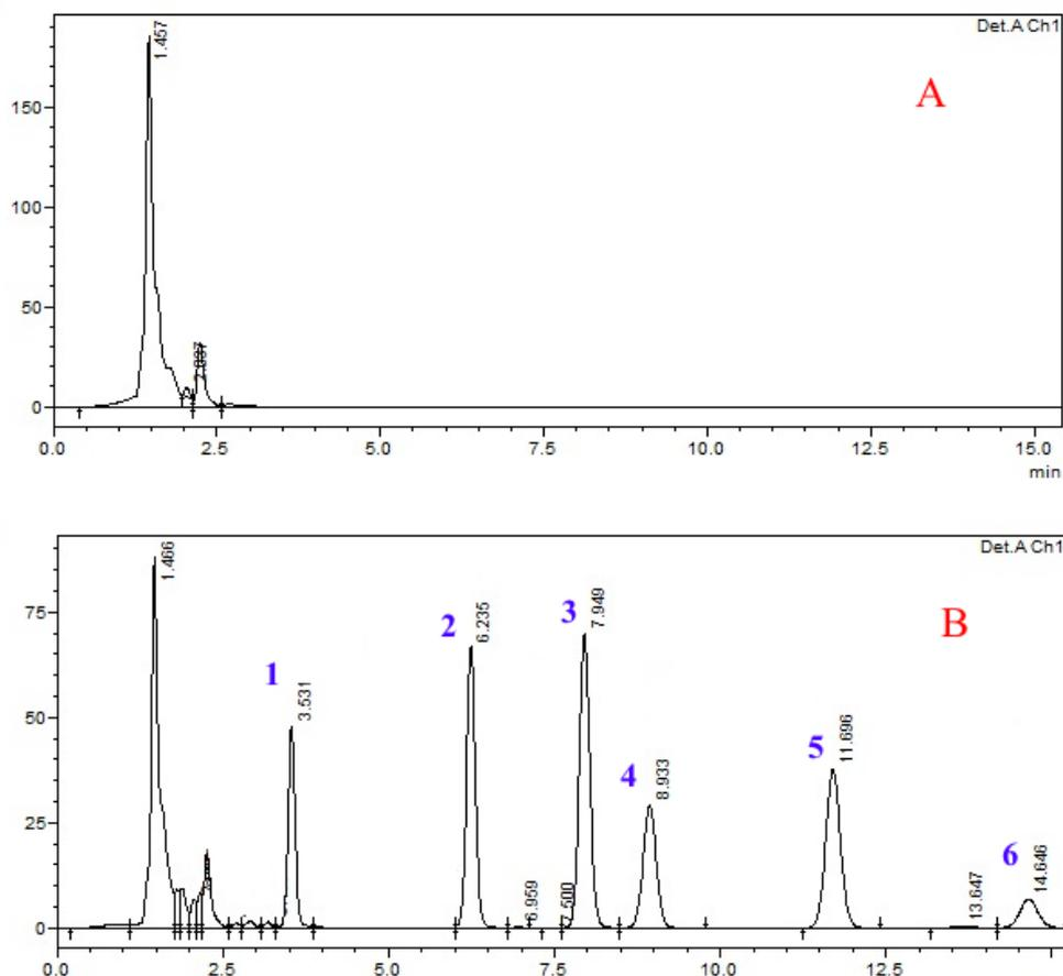
**Figure 4.** Typical chromatograms for blank human urine (A), human urine spiked with methicillin, dicloxacillin, nafcillin at  $8 \mu\text{g mL}^{-1}$ , oxacillin, cloxacillin at  $12 \mu\text{g mL}^{-1}$  and valsartan at  $0.8 \mu\text{g mL}^{-1}$  (B)
