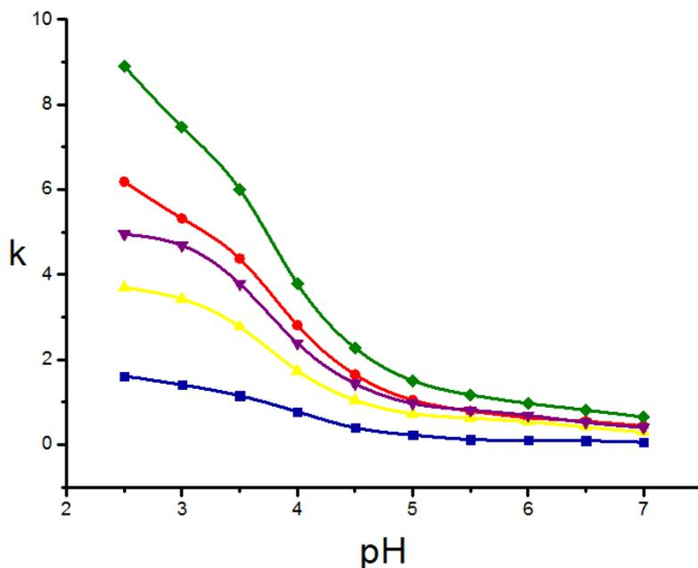
**Figure 2.** The effect of the mobile phase pH on retention factor values (40%, v/v) of acetonitrile: (■), methicillin; (●), nafcillin; (▲), oxacillin; (▼), cloxacillin; (◆), dicloxacillin. The theoretical results are indicated as continuous lines and the plotted points are experimental results
