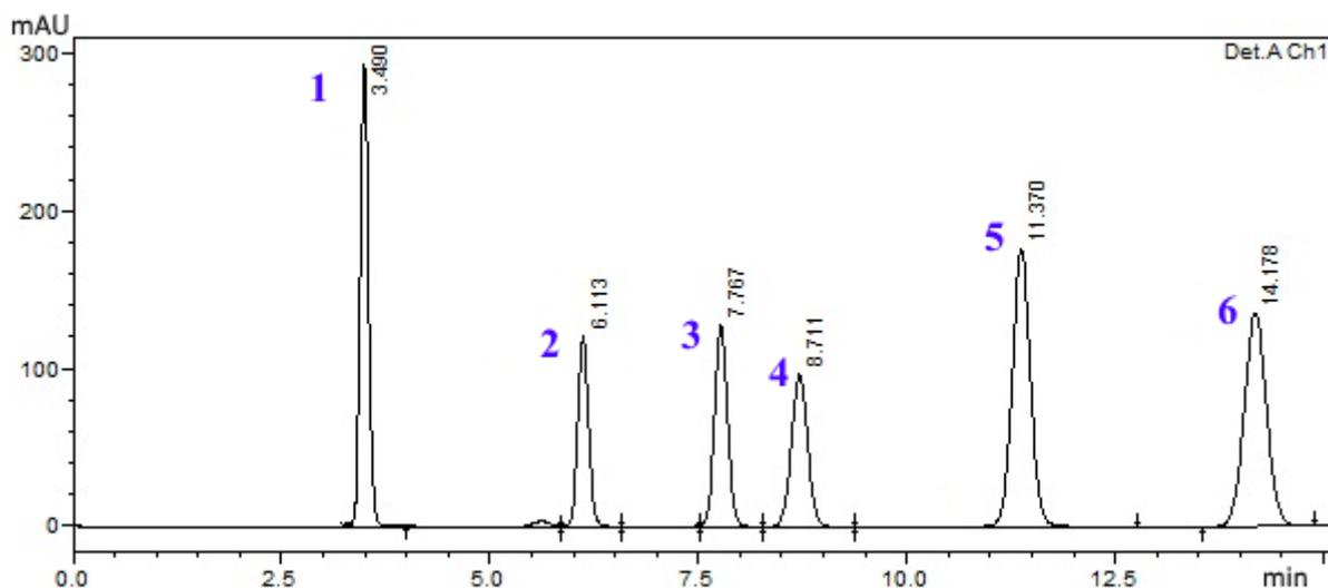
**Figure 3.** Optimized chromatogram of standard mixture. 1, methicillin ( $16,67 \mu\text{g mL}^{-1}$ ); 2, oxacillin ( $16,67 \mu\text{g mL}^{-1}$ ); 3, cloxacillin ( $16,67 \mu\text{g mL}^{-1}$ ); 4, nafcillin ( $16,67 \mu\text{g mL}^{-1}$ ); 5, dicloxacillin ( $16,67 \mu\text{g mL}^{-1}$ ); 6, valsartan (I.S.) ( $16,67 \mu\text{g mL}^{-1}$ ). Experimental conditions as in chromatographic procedure
