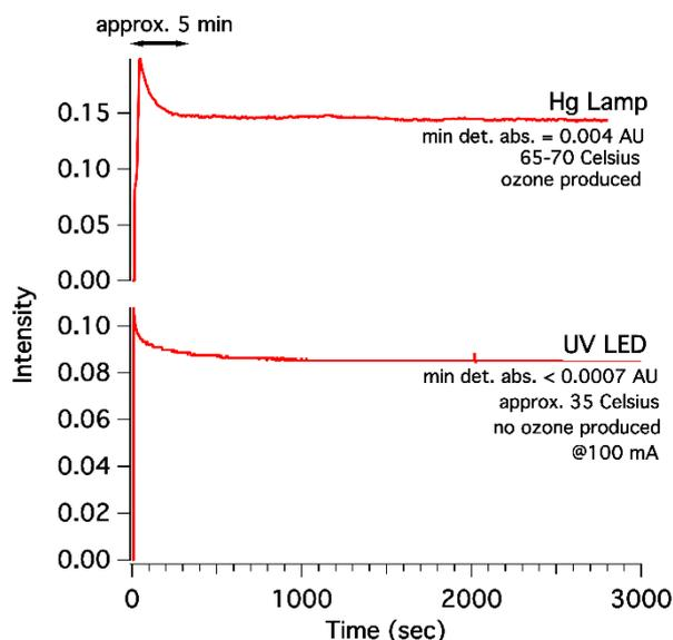
**Figure 2.** Comparison of the stability of a mercury lamp and the UV LED after power up
