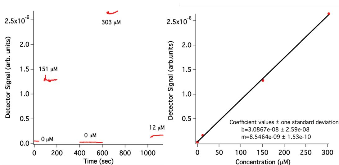
**Figure 3.** Calibration of the absorbance detector
