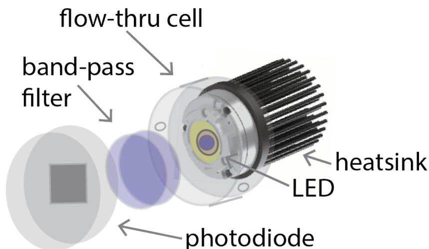
**Figure 1.** Illustration of LED based absorbance detector at 254 nm
