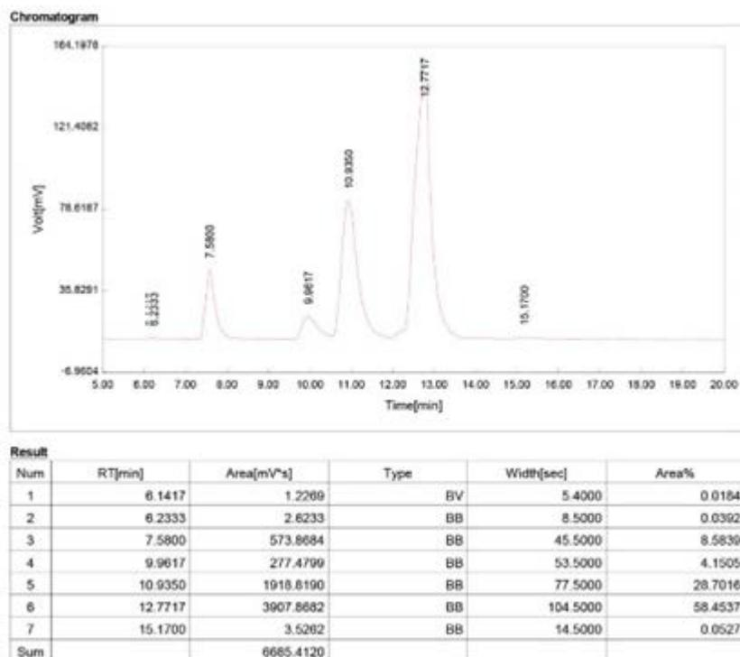
As the ester input has been given to the device, some peaks will be given to us. These diagrams would be analyzed by the device. Results show that all the samples contain the desirable mixtures. However the length & width of the peaks were different in the chromatograph, but it showed that the maximum amount is related to C18:2.
