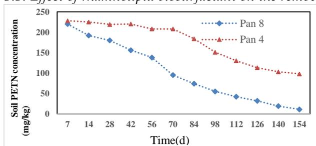
**Fig.3:** effect of rhamnolipid on bioremediation of PETN. Pan 4 amended with sludge. Pan 8 amended with rhamnolipid plus sludge.
