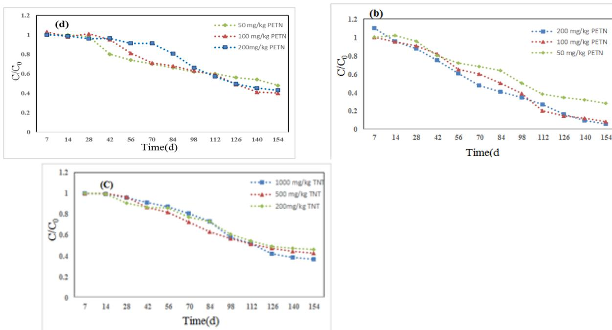
**Fig.1:** Disappearance of TNT and PETN with time by addition of rhamnolipid (a), (b) and without addition of rhamnolipid (c), (d)
