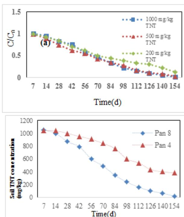
**Fig.2:** Effect of rhamnolipid on bioremediation of TNT. Pan 4 amended with sludge. Pan 8 amended with rhamnolipid plus sludge.
