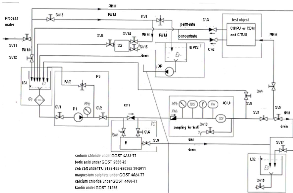
**Figure 4.** Hydraulic circuit of the test bench:
