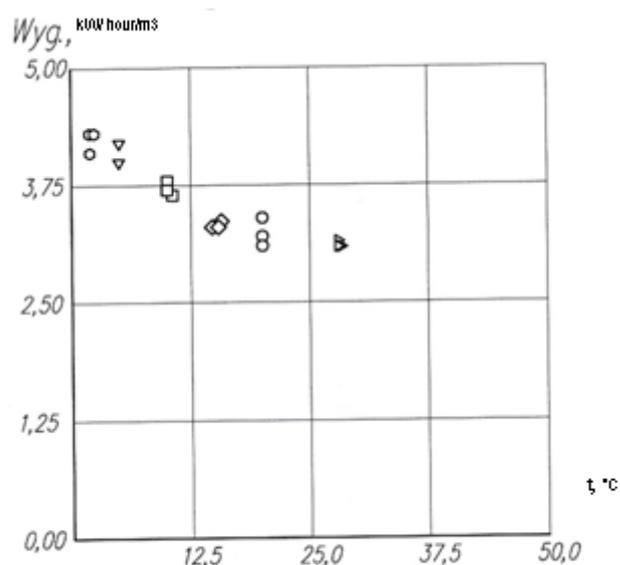
**Figure 5.** Dependence of specific energy consumption by the RODM ( $W_{sp}$ ,  $KWh/m^3$ ) on source water temperature ( $t$ ,  $^{\circ}C$ )
