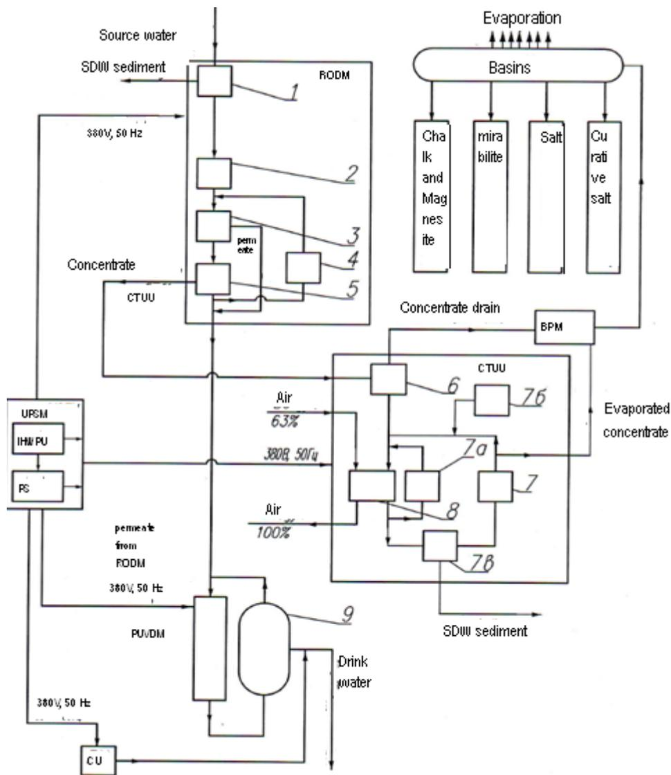
**Figure 1.** Flowchart of an experimental sample of the combined wind power unit:
