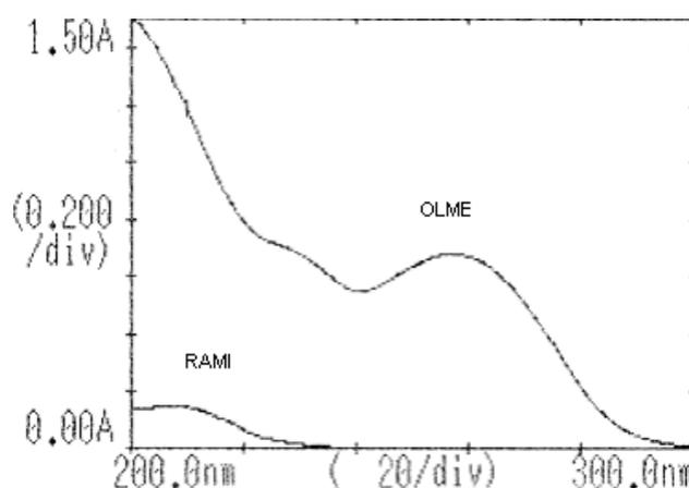
**Figure 3.** Overlay spectrum of ramipril and olmesartan medoxomil in water: acetonitrile (50:50). RAMI ( $4 \mu\text{g}\cdot\text{mL}^{-1}$ ) is ramipril, OLME is olmesartan medoxomil ( $16 \mu\text{g}\cdot\text{mL}^{-1}$ ) taken on UV-Vis spectrophotometer. (Shimadzu 1700).
