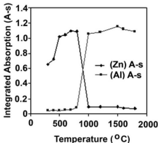
**Fig.3.** Optimization of the pyrolysis temperature of Aluminum and Zinc
