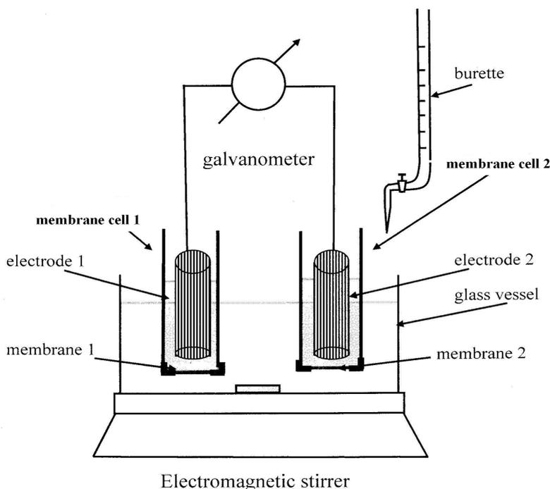
**Fig.1.** Experimental setup for Dialysis amperometry.
