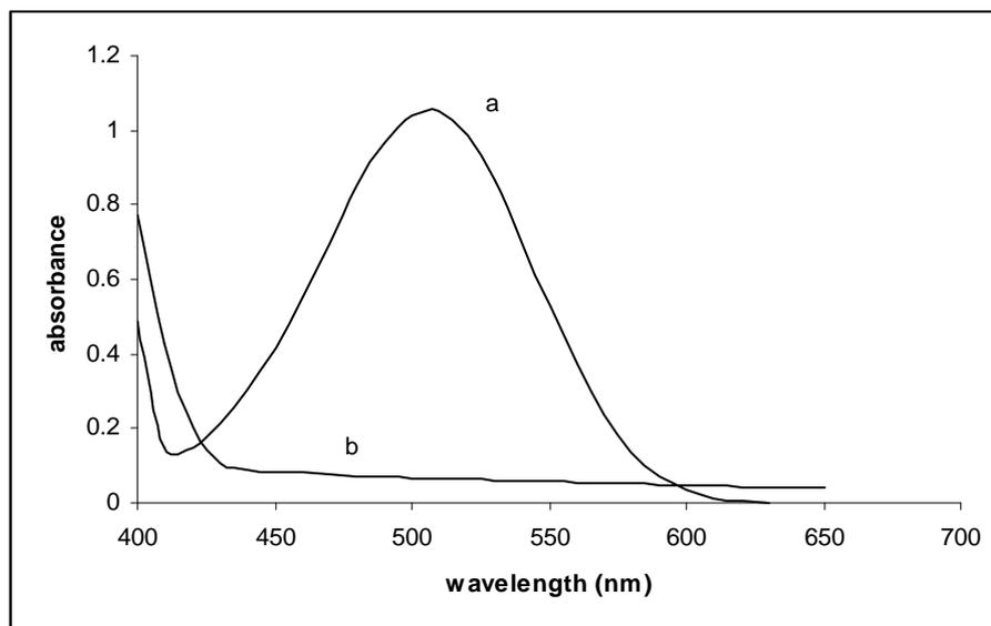
**Fig. 2.** (a) The absorption spectrum of the PDAB-RNH condensation product (b) corresponding reagent blank.
