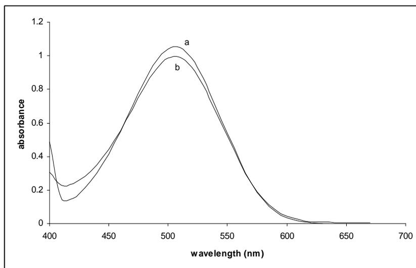
**Fig. 3.** (a) The absorption spectrum as soon as the product formed (b) absorption spectrum of the product after 10 hrs.
