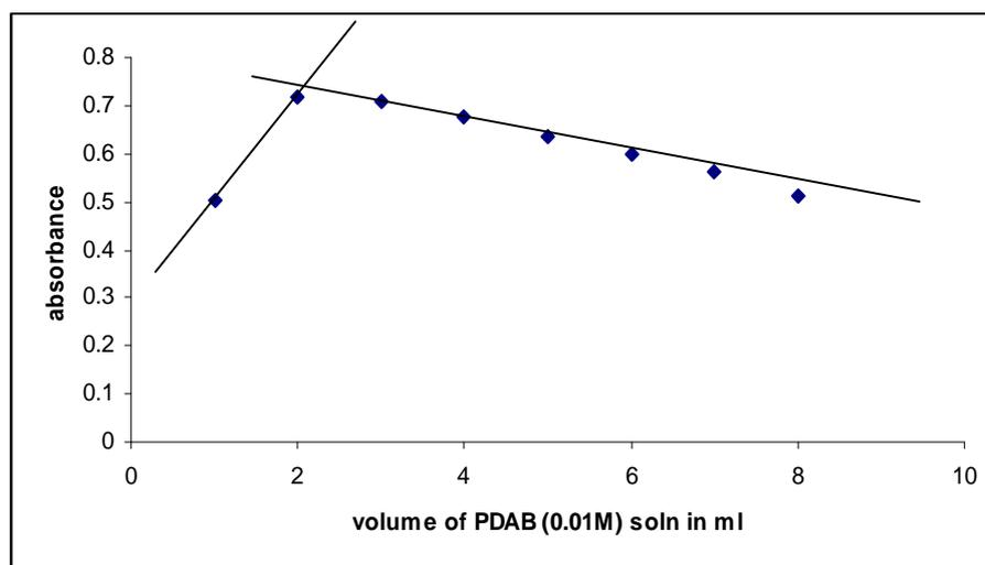
**Fig. 4.** Mole-ratio method to determine the stoichiometric relationship between PDAB and RNH
