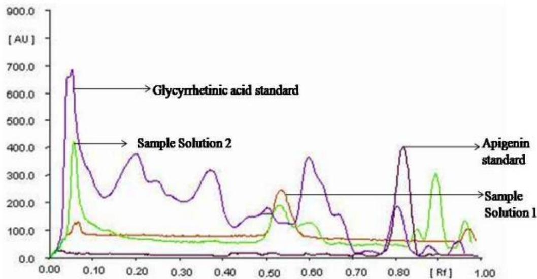
**Fig. 4:** TLC densitometric scan at 254 nm of test solutions and standard solutions of *Glycyrrhiza glabra* roots and rhizomes
