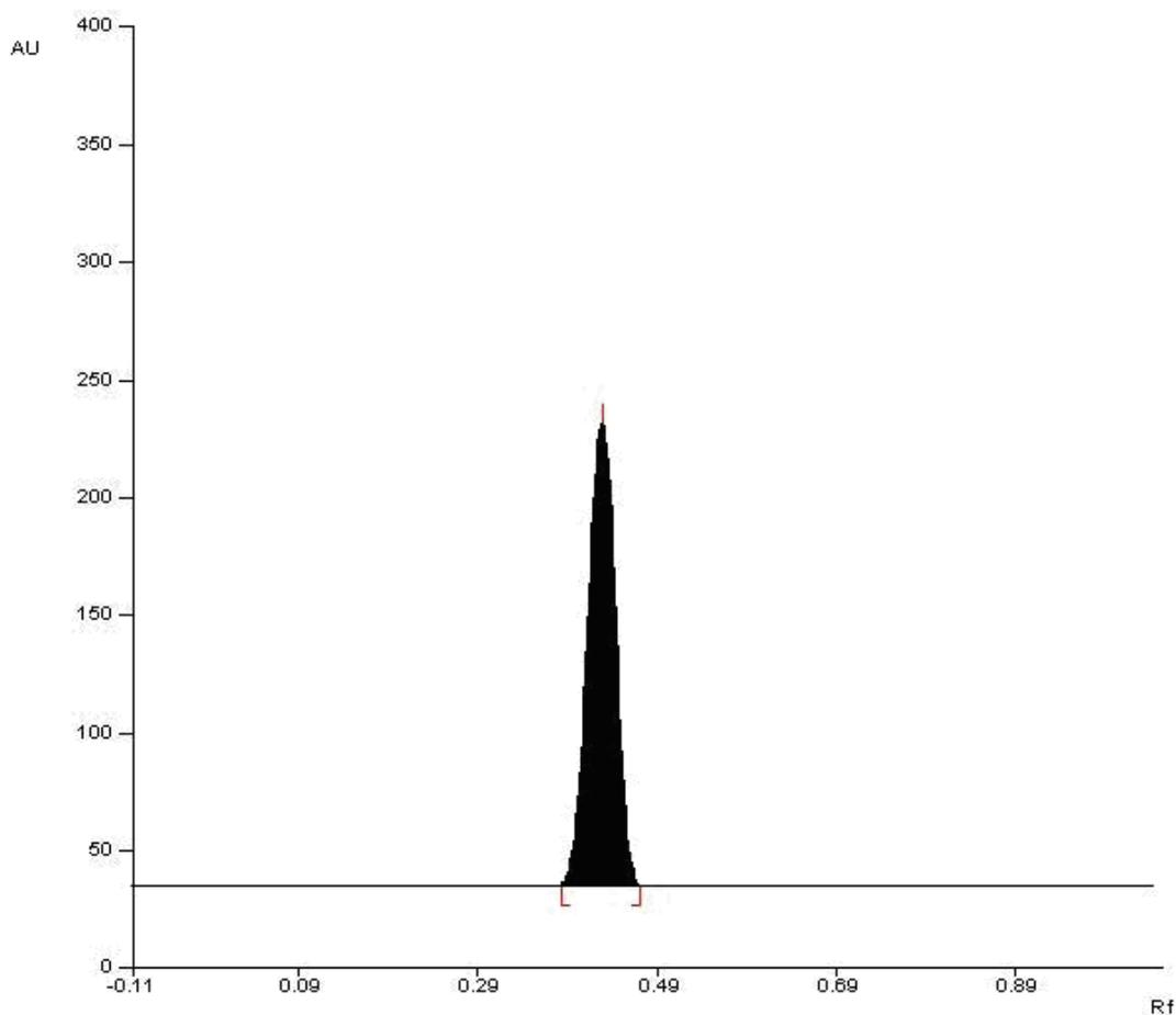
**Fig. 2.** Chromatogram of rabeprazole sodium in mobile phase acetone: water (3.5: 1.5 v/v with  $R_f = 0.45$ )
