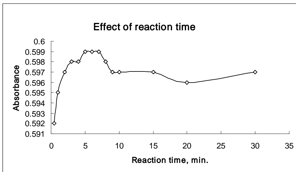
Fig.5 The effect of the complex formation equilibrium time on the absorbance of Mg(II)-EBT complex in surfactant medium at 640 nm and at pH: 9.5 under optimum conditions
