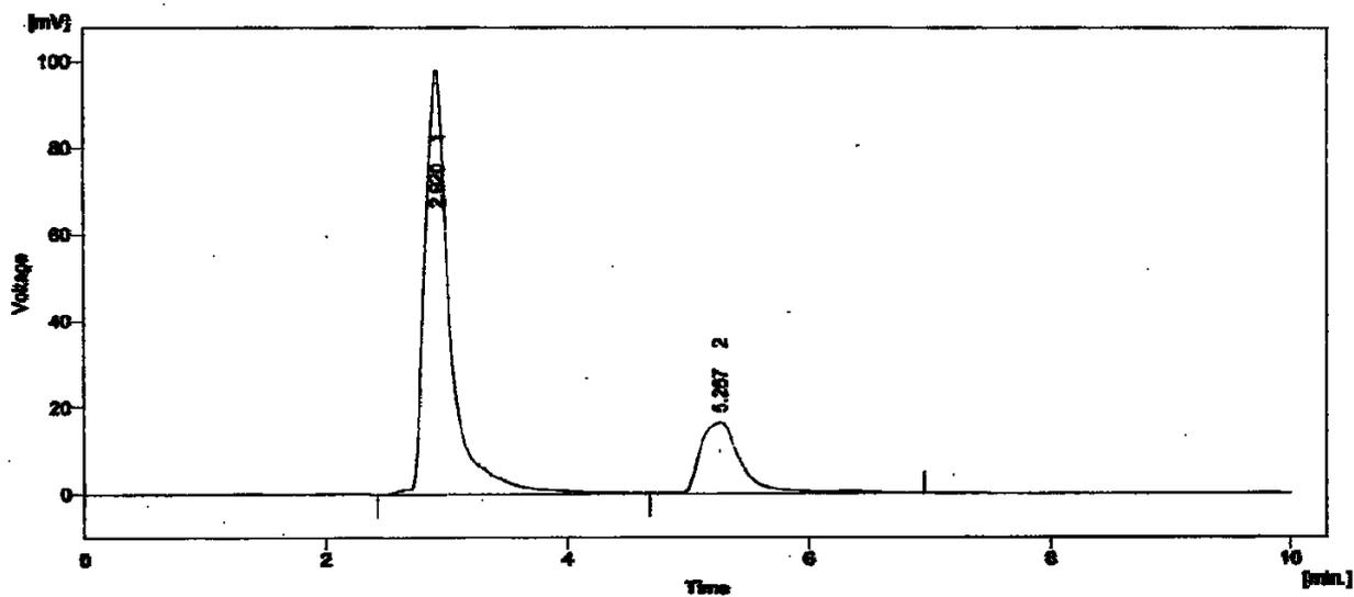
**Fig. 2a.** Chromatograms of alkali degraded sample: 1) NTA, 2) ATR
