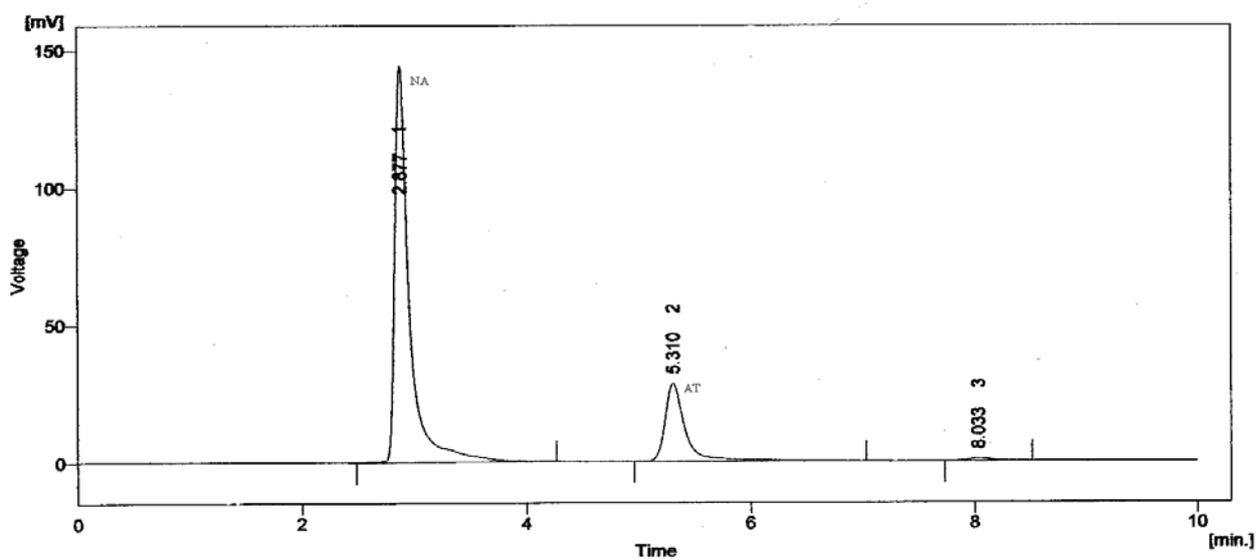
**Fig. 1.** Chromatogram of untreated marketed formulation: 1) NTA, 2) ATR
