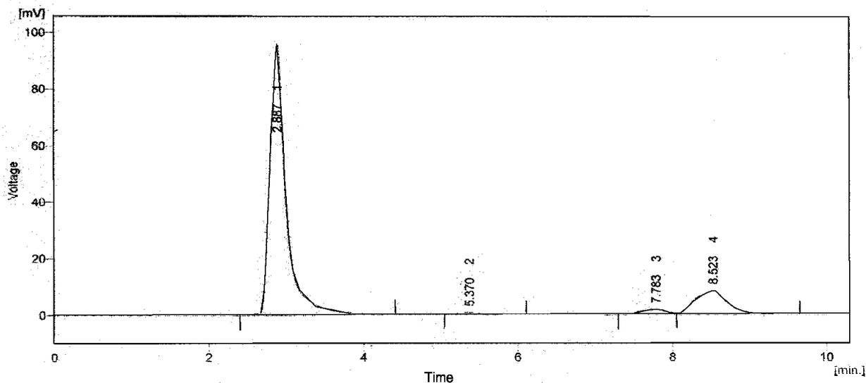
**Fig. 2b.** Chromatogram of Acid degraded sample
