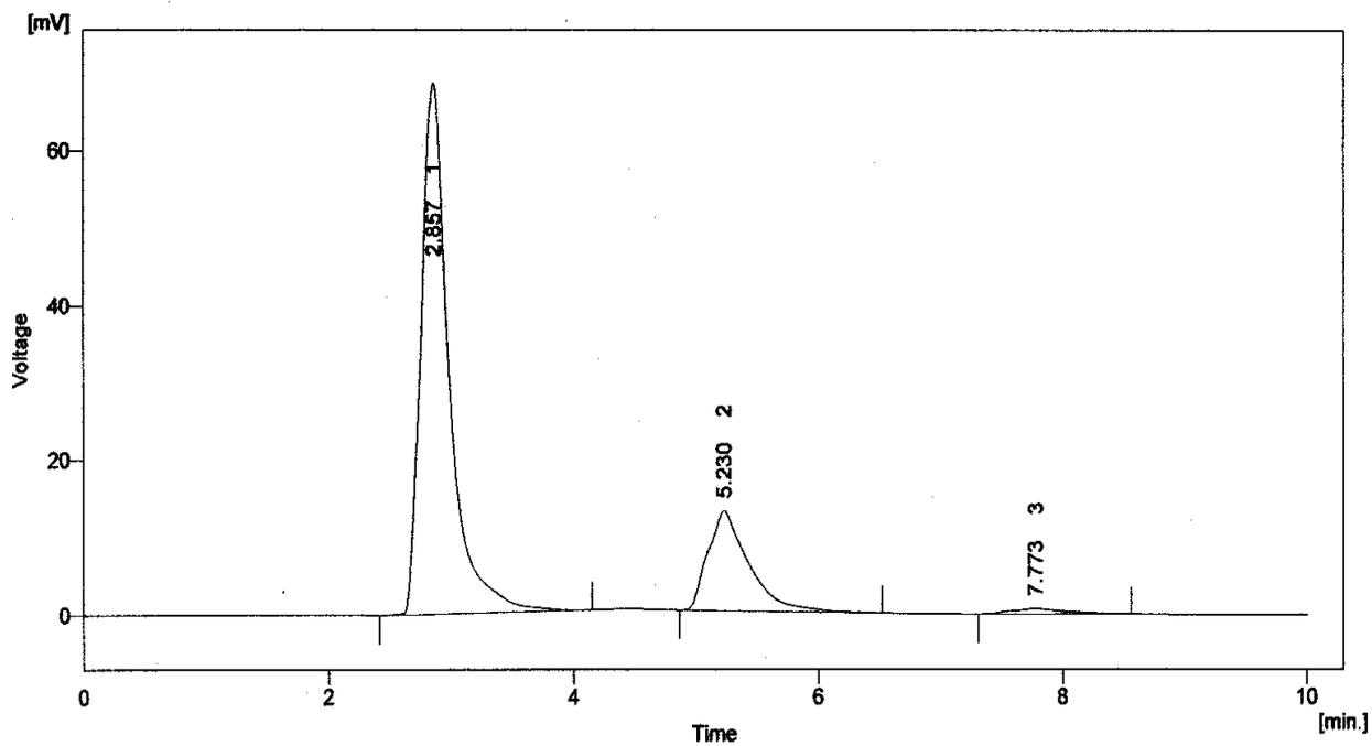
**Fig. 2e.** Chromatogram of Humidity degraded sample- 1) NTA 2) ATR
