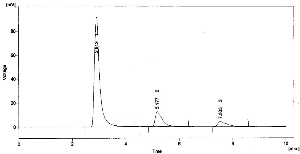
**Fig. 2d.** Chromatogram of Thermal degraded sample 1) NTA 2) ATR 3) ATR degraded product
