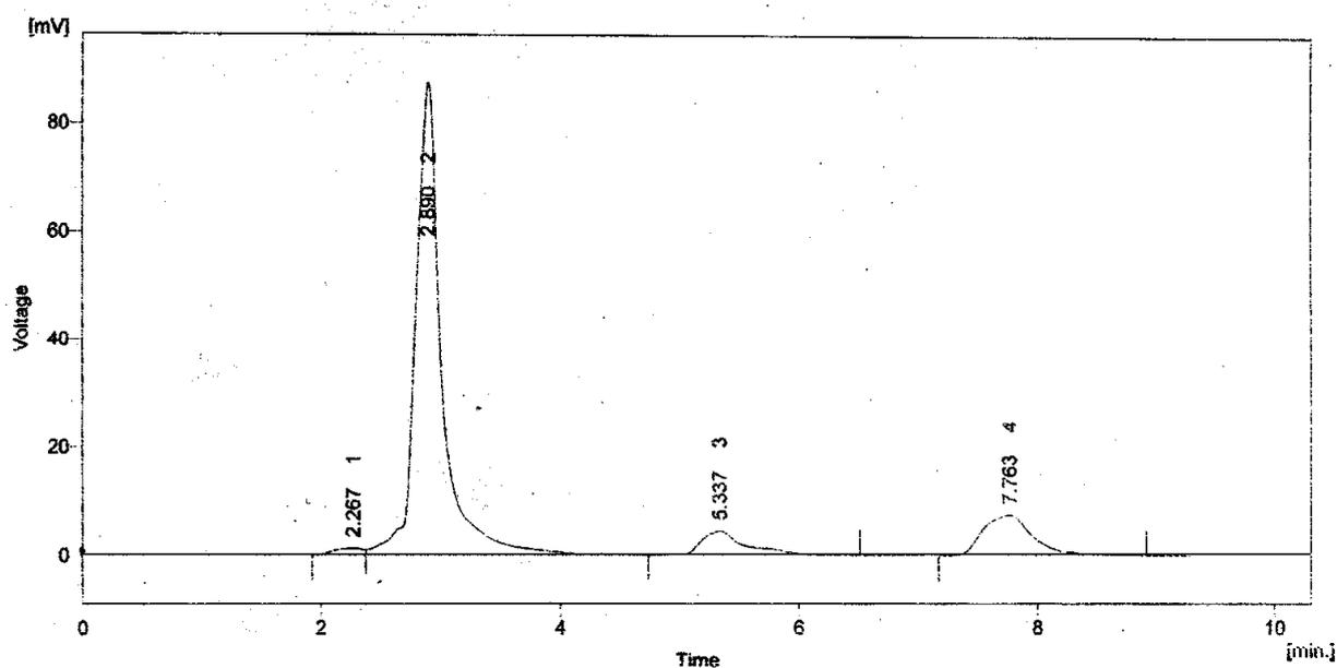
**Fig. 2c.** Chromatogram of oxide degraded sample 2) NTA 3) ATR 4) ATR degraded product
