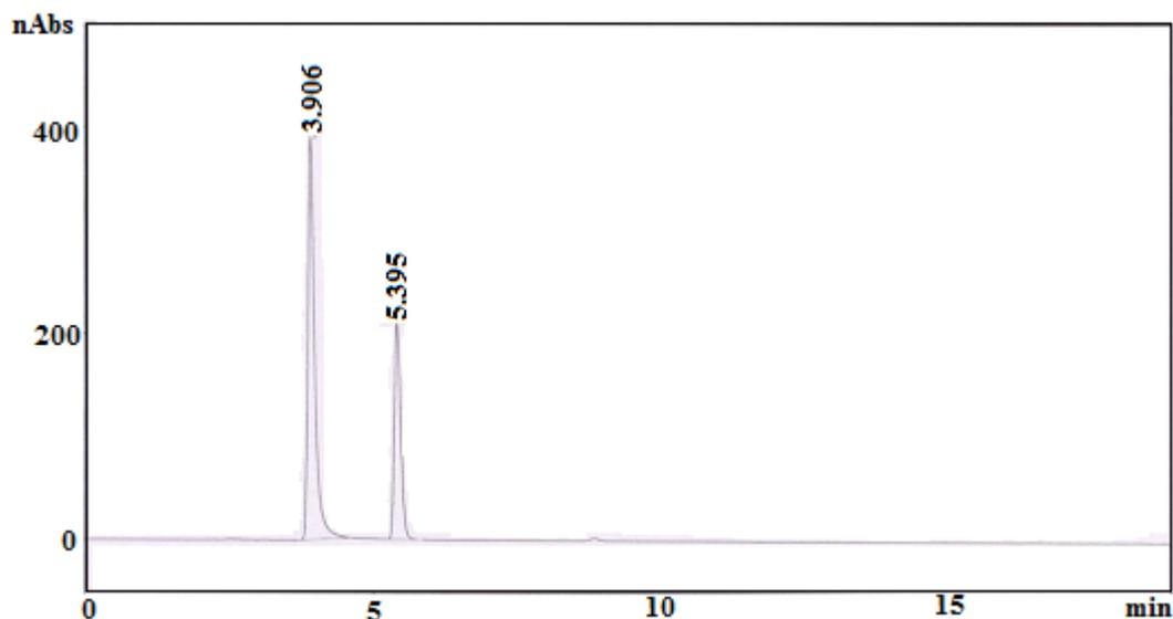
**Fig.3.** A typical chromatogram of the tablet: ofloxacin (3.9 min), and nitazoxanide (6.36 min)
