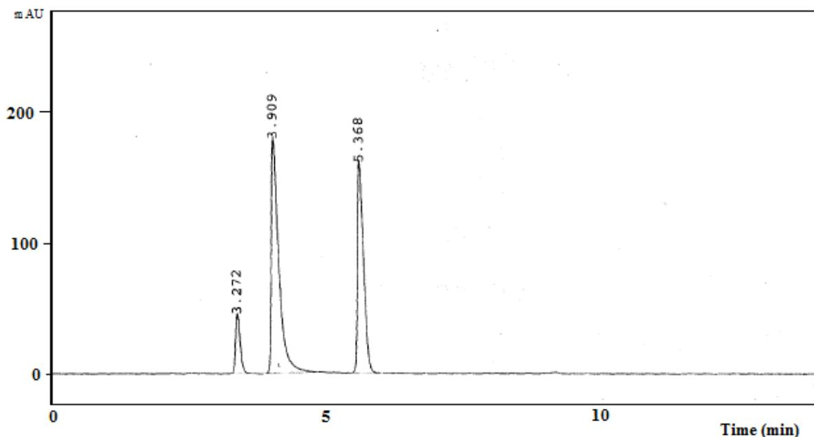
**Fig. 2.** A typical chromatogram of the tablet: caffeine (3.27 min ), ofloxacin (3.9 min), and nitazoxanide (6.36 min)
