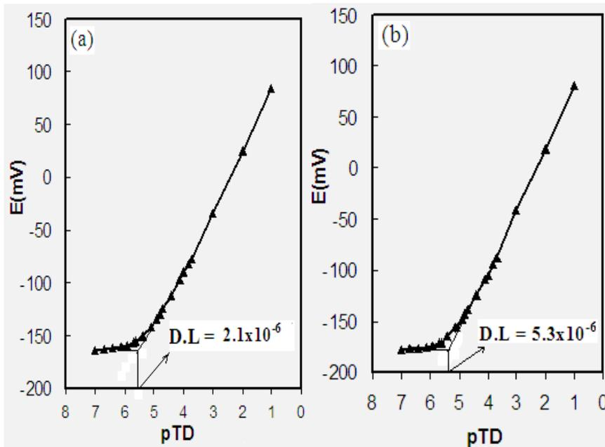
**Fig. 2.** The calibration curve and the detection limit value for electrodes a) TD-ST b) TD-SM
