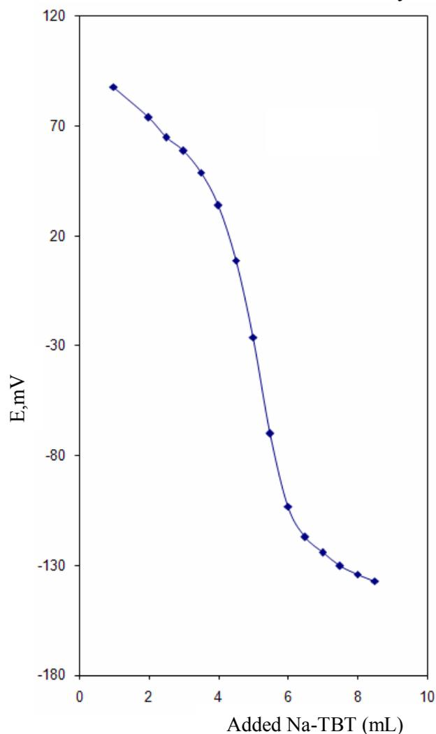
**Fig. 5.** Potentiometric titration of 5.0 mL of  $1.0 \times 10^{-2} \text{ mol L}^{-1}$  TDCI with  $1.0 \times 10^{-2} \text{ mol L}^{-1}$  Na-TPB as a titrant using TD.ST electrode
