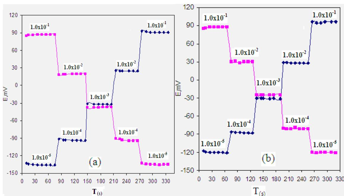
**Fig. 3.** Dynamic response time of (a) TD-ST electrode and (b) TD-SM electrode for step changes in concentration of TDCI (from low to high and vice versa)
