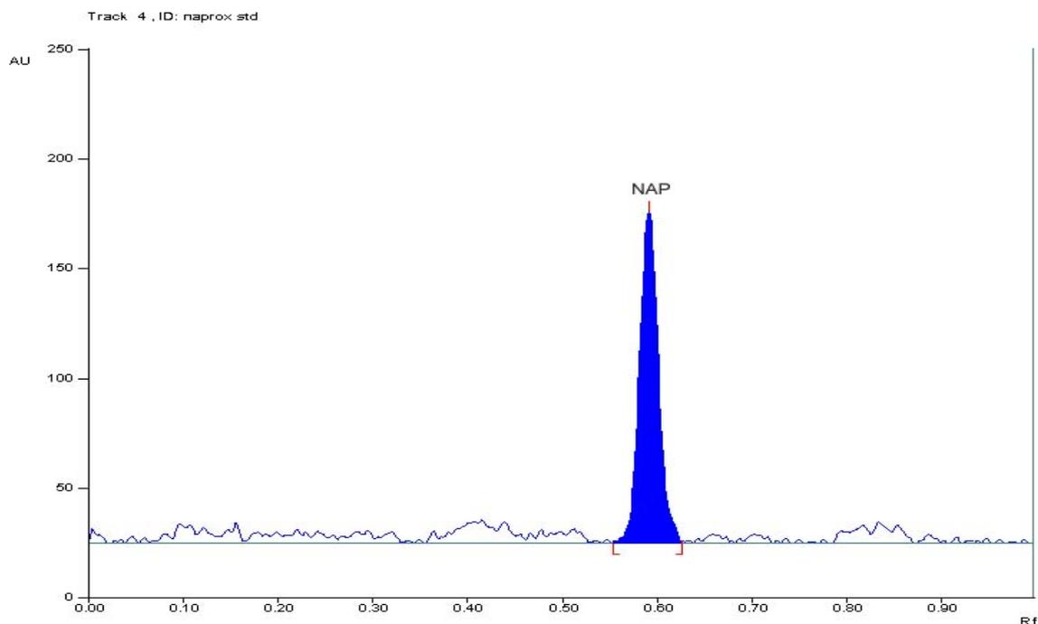
**Fig. 1** Densitogram of Naproxen sodium (200 ng band<sup>-1</sup>, Rf = 0.63  $\pm$  0.013)
