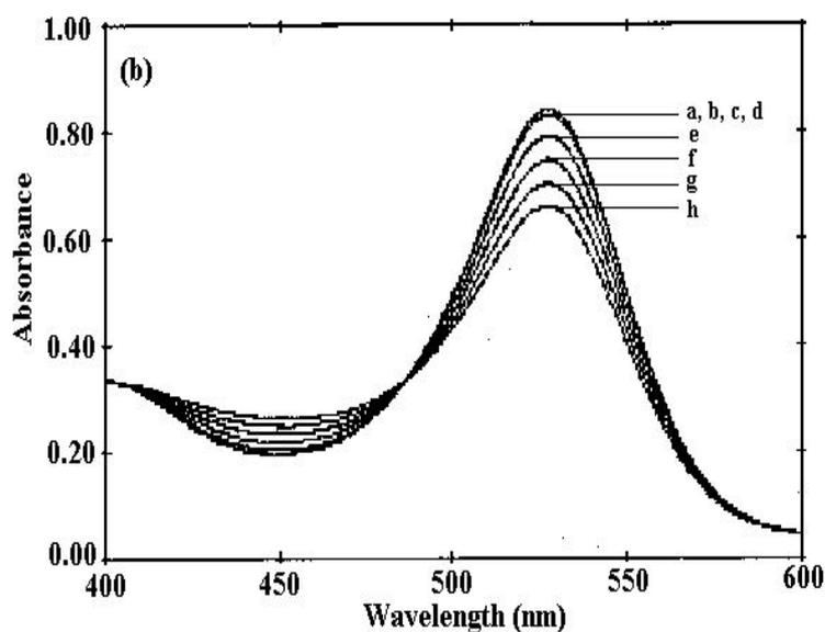
**Fig 1b.** Absorption spectra of reaction system in the presence of  $1.0 \text{ } \mu\text{g mL}^{-1}$  As(III). Conditions: same as Fig 1a.
