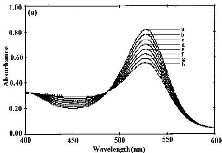
**Fig 1a.** Absorption spectra of reaction system in the absence of As(III). Conditions: HCl,  $0.10 \text{ mol L}^{-1}$ ; MCP,  $2.6 \times 10^{-5} \text{ mol L}^{-1}$ ; NaIO<sub>4</sub>,  $3.5 \times 10^{-3} \text{ mol L}^{-1}$ ; KBr,  $2.2 \times 10^{-3} \text{ mol L}^{-1}$  and temperature of  $20.0 \text{ }^\circ\text{C}$  with scan time intervals of 15 s.
