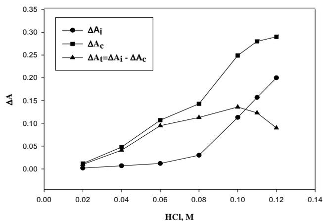
**Fig 3.** Effect of HCl concentration. Conditions: MCP,  $2.6 \times 10^{-5} \text{ mol L}^{-1}$ ;  $\text{NaIO}_4$ ,  $2.5 \times 10^{-3} \text{ mol L}^{-1}$ ; KBr,  $2.00 \times 10^{-3}$ ; As(III),  $1.0 \mu\text{g mL}^{-1}$  and temperature of  $20.0 \text{ }^\circ\text{C}$ .
