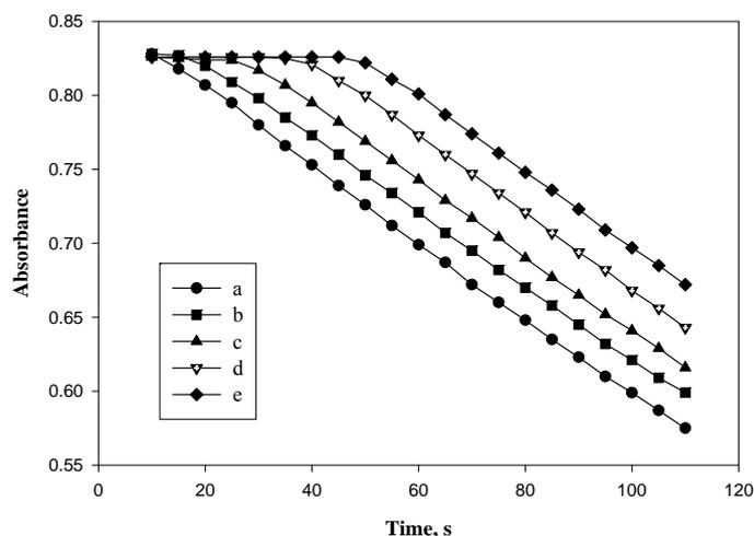
**Fig 2.** Absorbance change profile. Conditions: Same as Fig. 1a with As(III) concentrations of (a) 0.00, (b) 0.20, (c) 0.40, (d) 0.60 and (e) 0.80  $\mu\text{g mL}^{-1}$ .
