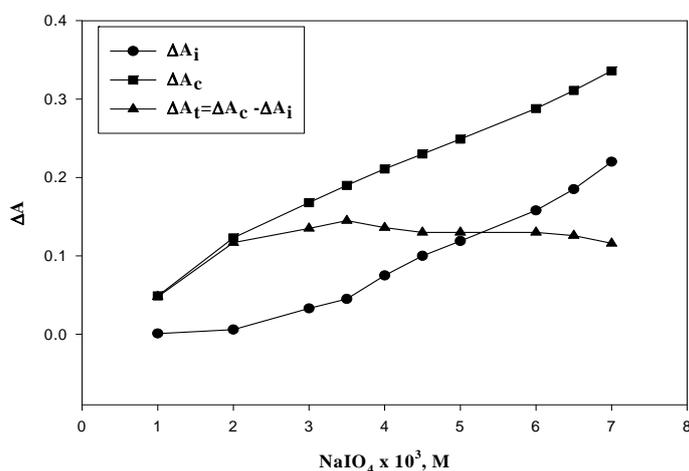
**Fig 4.** Effect of sodium periodate concentration. Conditions: HCl,  $0.10 \text{ mol L}^{-1}$ ; MCP,  $2.6 \times 10^{-5} \text{ mol L}^{-1}$ ; KBr,  $2.00 \times 10^{-3} \text{ mol L}^{-1}$ ; As(III),  $1.0 \mu\text{g mL}^{-1}$  and temperature of  $20.0 \text{ }^\circ\text{C}$
