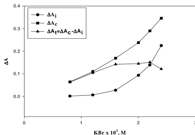
**Fig 5.** Effect of potassium bromide concentration. Conditions: HCl, 0.10 mol L<sup>-1</sup>; MCP, 2.6×10<sup>-5</sup> mol L<sup>-1</sup>; NaIO<sub>4</sub>, 3.5×10<sup>-3</sup> mol L<sup>-1</sup>; As(III), 1.0 μg mL<sup>-1</sup> and temperature of 20.0 °C.
