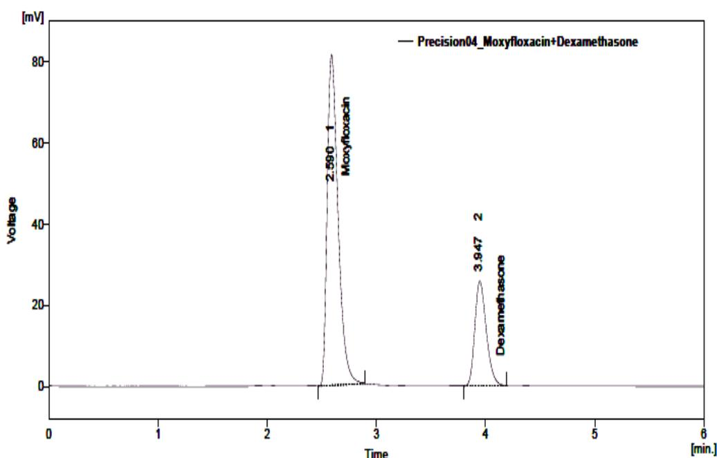
**Fig. 1.** Typical chromatogram for the standard solution of MFN and DSP
