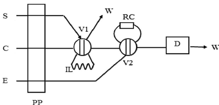
**Fig. 2:** FI manifold proposed for the continuous determination of hexazinone in water: sample solution (S), carrier solution (C), eluent (E), peristaltic pump (PP), injection valves 1 and 2 (V), injection loop (IL), retention column (RC), detector (D), and wastes (W).
