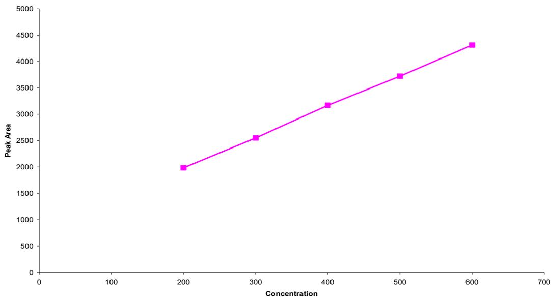
**Figure 7.** Calibration curve of atorvastatin calcium
