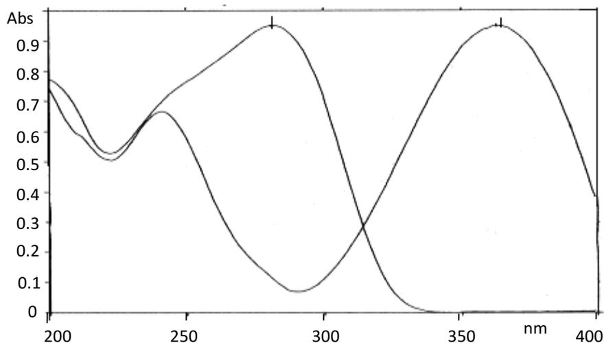
**Figure 3:** UV spectra of standard atorvastatin calcium and standard amlodipine besylate on TLC plate
