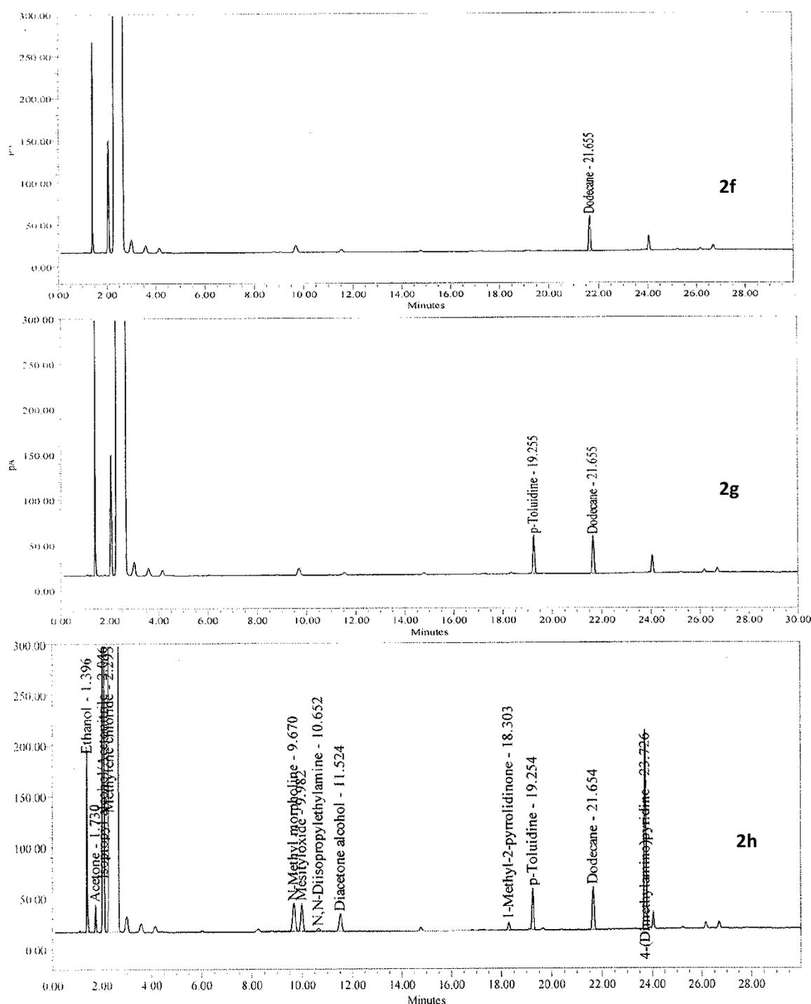
**Fig. 2.** Typical GC chromatograms of 2(f) Chromatogram of IMP drug substance, 2(g) Chromatogram of IMP drug substance spiked with *p*-Toluidine and 2(h) Chromatogram of IMP drug substance spiked with *p*-Toluidine including other known residual solvents
