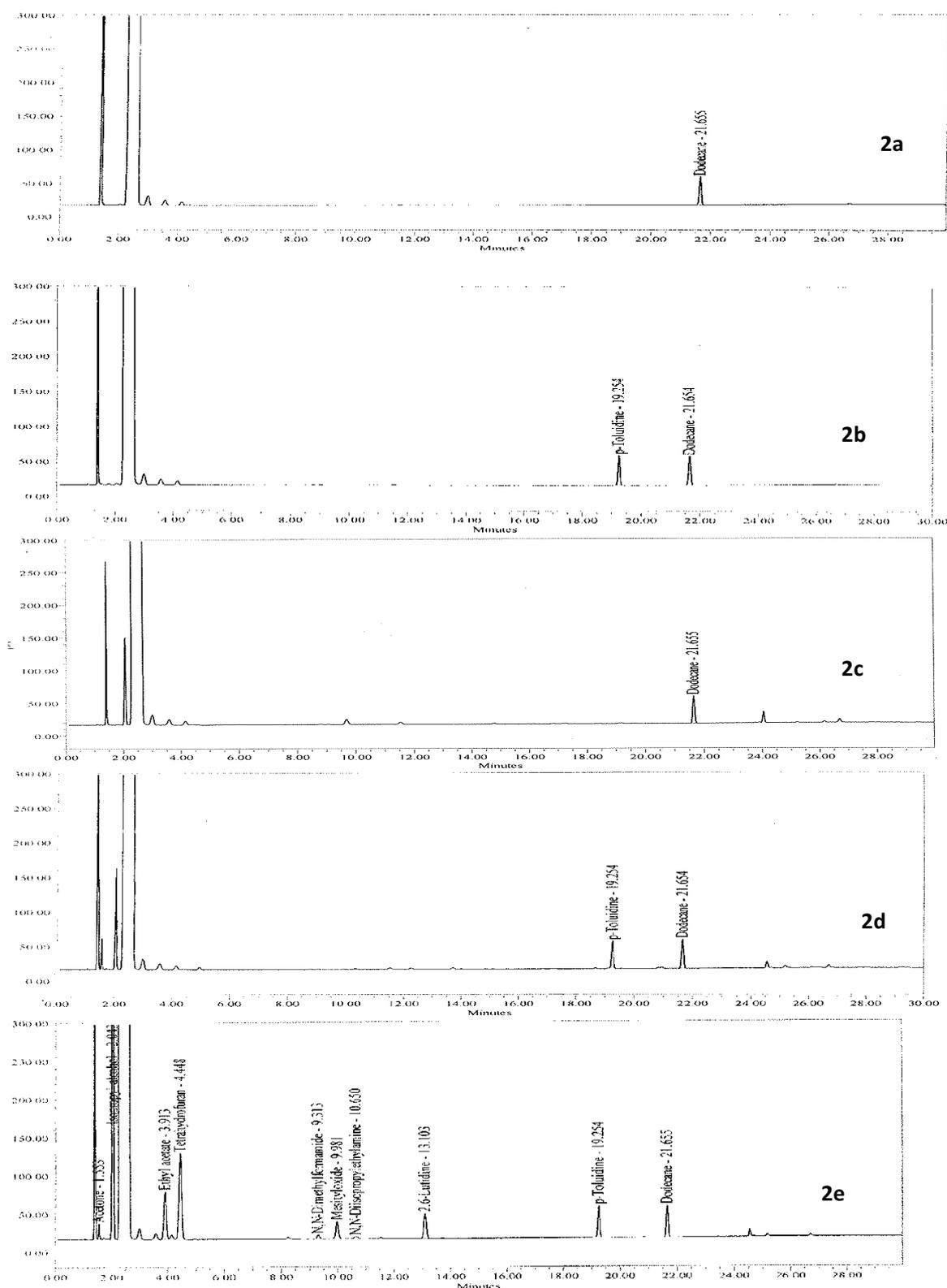
**Figure 2.** Typical GC chromatograms of 2(a) Chromatogram of Blank, 2(b) Chromatogram of Standard. 2(c) Chromatogram of MER drug substance, 2(d) Chromatogram of MER drug substance spiked with *p*-Toluidine and 2(e) Chromatogram of MER drug substance spiked with *p*-Toluidine including other known residual solvents
