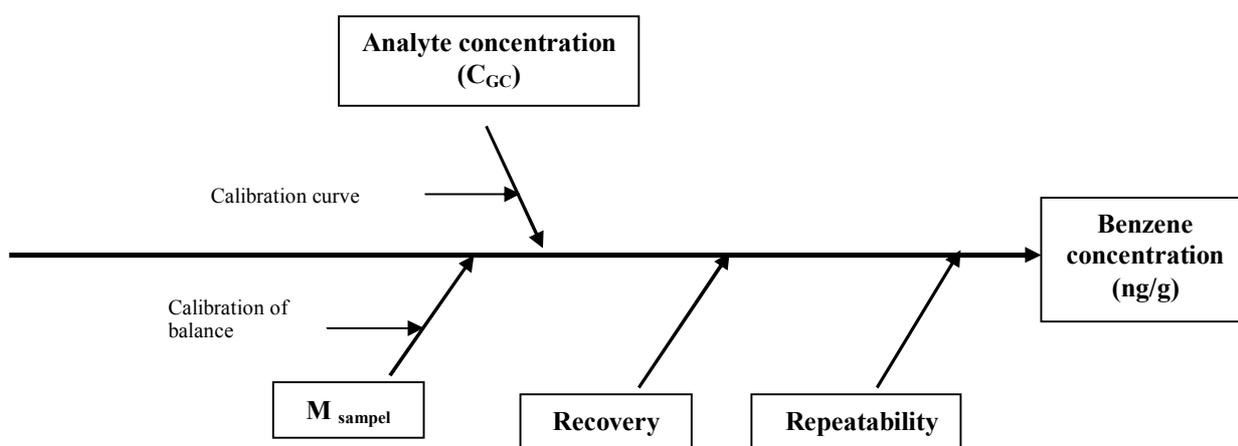
**Fig.5** Cause and effect diagram for determination of Benzene in drinking water and beverages samples.
