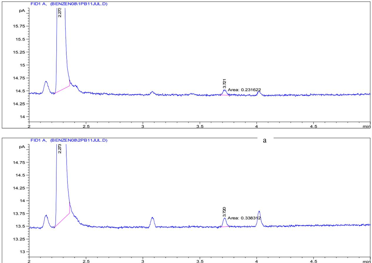
**Fig.3** A chromatogram of benzene in the aquadest at concentration of a)  $1 \text{ ng mL}^{-1}$ ; b)  $2 \text{ ng mL}^{-1}$
