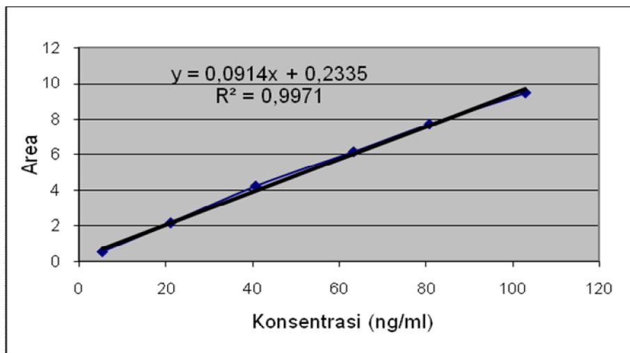
**Fig. 2.** Calibration curve of benzene in aquadest with the linear range from 5-100 ng mL<sup>-1</sup>.
