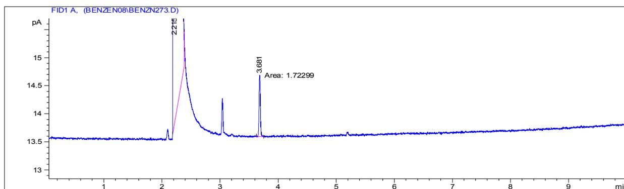
**Fig. 1.** Chromatogram of standard benzene in the aquadest sample.
