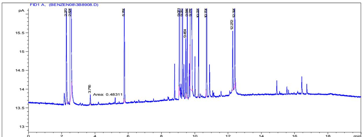
**Fig. 4.** The chromatogram resulted from the analysis of benzene at the concentration level of  $3.23 \text{ ng mL}^{-1}$  in the beverage sample.
