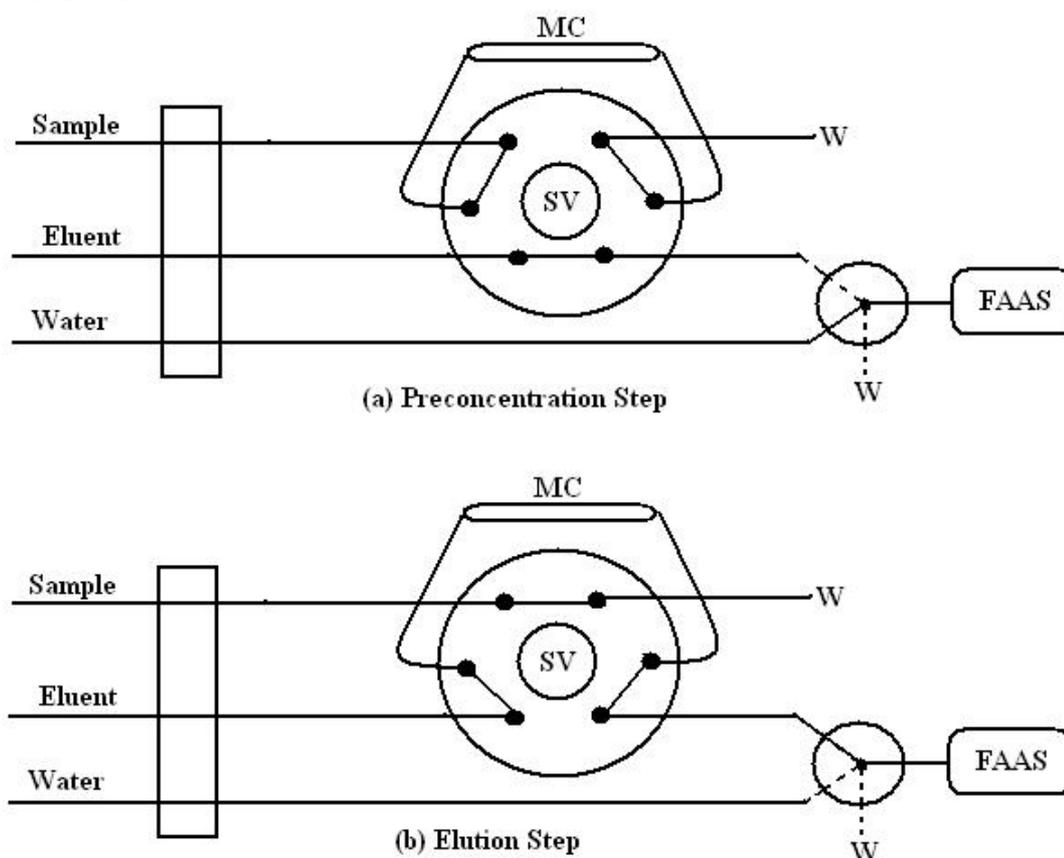
**Fig.2.** Schematic diagram of FI-manifold and the two operation sequences for copper(II) determination by FAAS.
