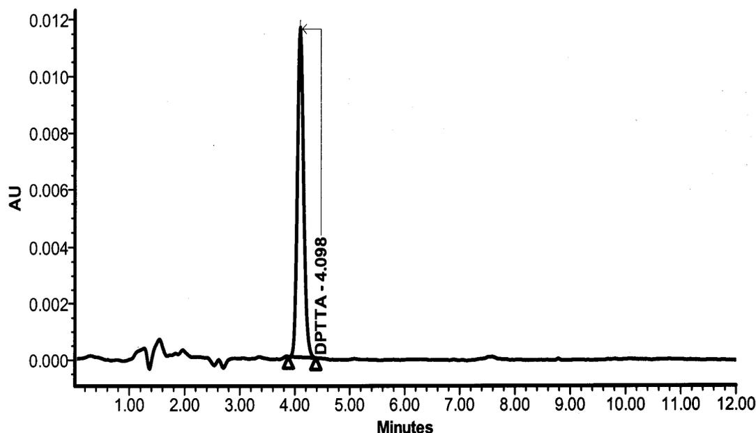
**Fig. 2.** Typical chromatogram of DPTTA standard
