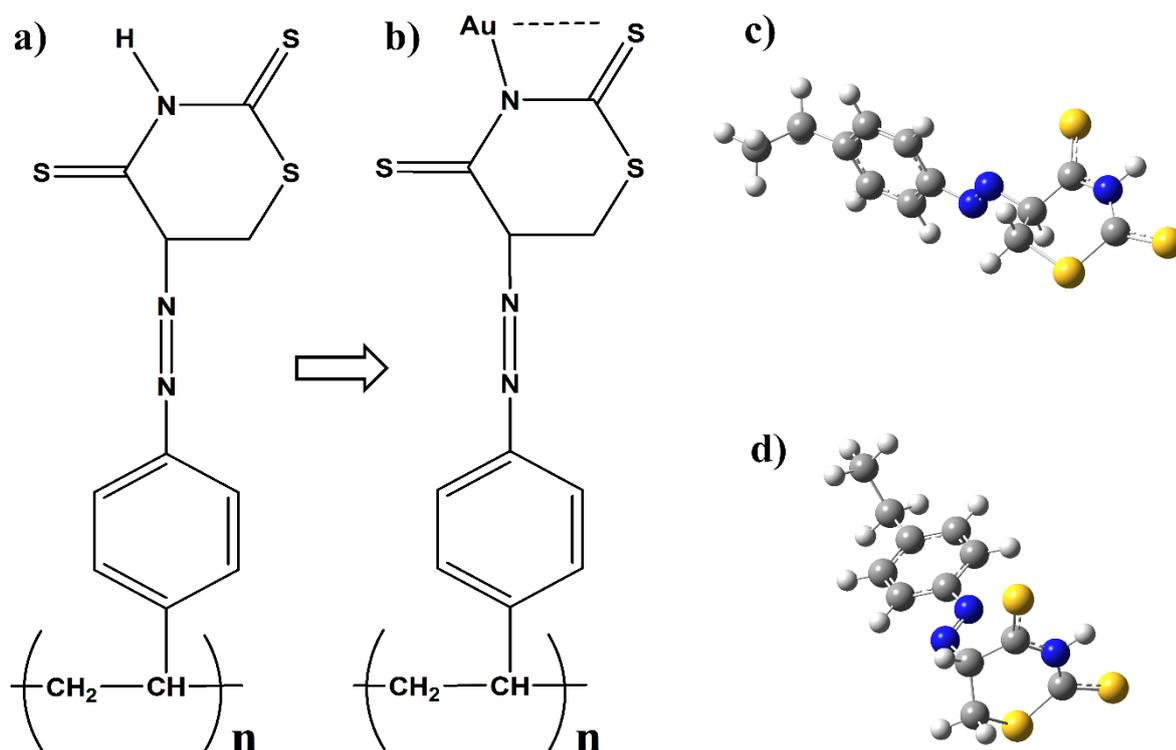
**Figure 1.** The PSTDT polymer without (a, c and d) and with (b) gold
