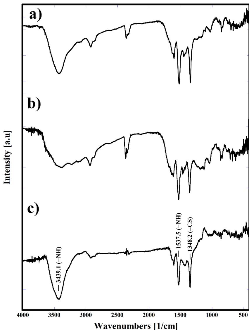
**Figure 3.** The IR spectra of PSTDT polymer with (a) and without (b) gold, and difference (c)
