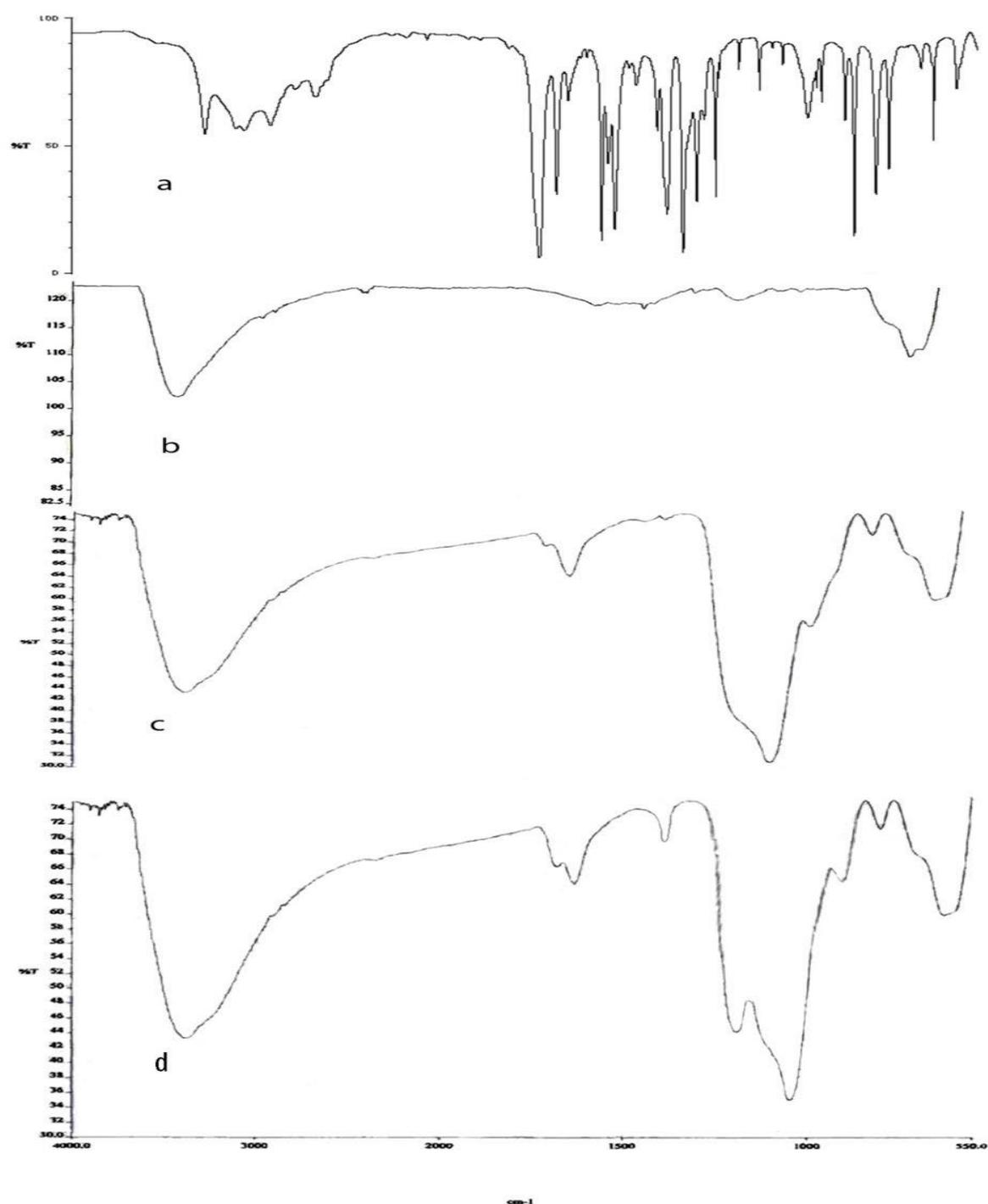
**Figure 5.** FT-IR spectra (a) SA (b) magnetic nanoparticles (c) SiO<sub>2</sub> coated magnetic nanoparticles (d) SiO<sub>2</sub> coated magnetic nanoparticles modified with SA [45]
