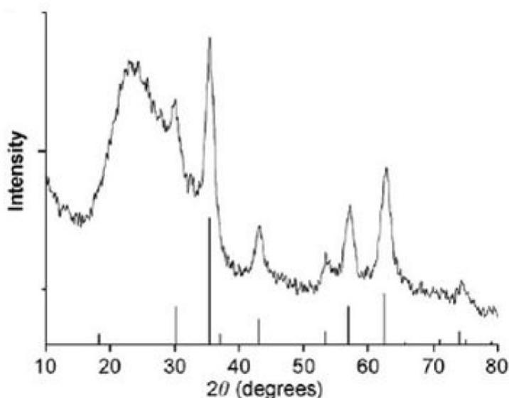
**Figure 4.** XRD pattern of silica-coated magnetic nanoparticles [45]
