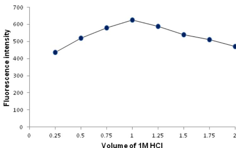
**Figure 8.** Effect of volume of 1M HCl on the fluorescence intensity of reaction product at  $\lambda_{em}$  543 nm
