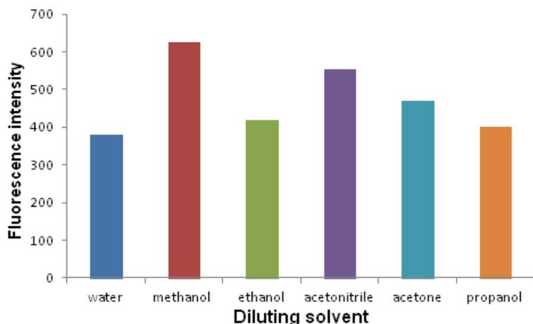
**Figure 9.** Effect of diluting solvent on the fluorescence intensity of reaction product at  $\lambda_{em}$  543 nm
