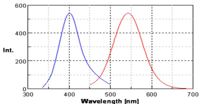
**Figure 3.** Excitation and emission spectra of the reaction product of oxymetazoline hydrochloride ( $7 \mu\text{g mL}^{-1}$ ) with 0.1% NBD-Cl
