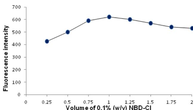
**Figure 4.** Effect of volume of 0.1% NBD-Cl on the fluorescence intensity of reaction product at  $\lambda_{em}$  54 nm
