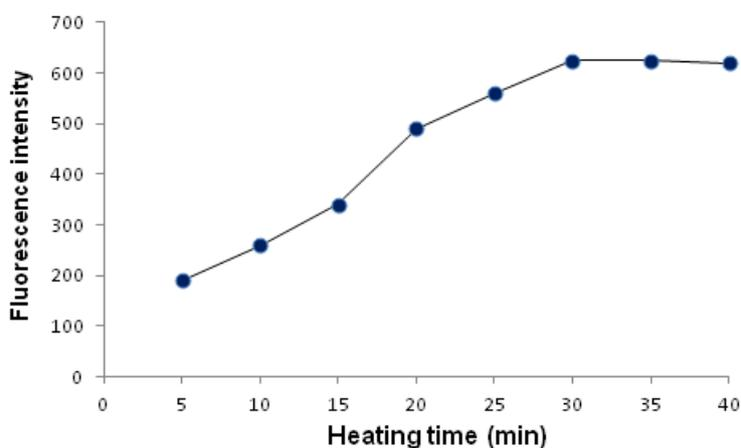
**Figure 7.** Effect of heating time at 60 °C on the fluorescence intensity of reaction product at  $\lambda_{em}$  543nm
