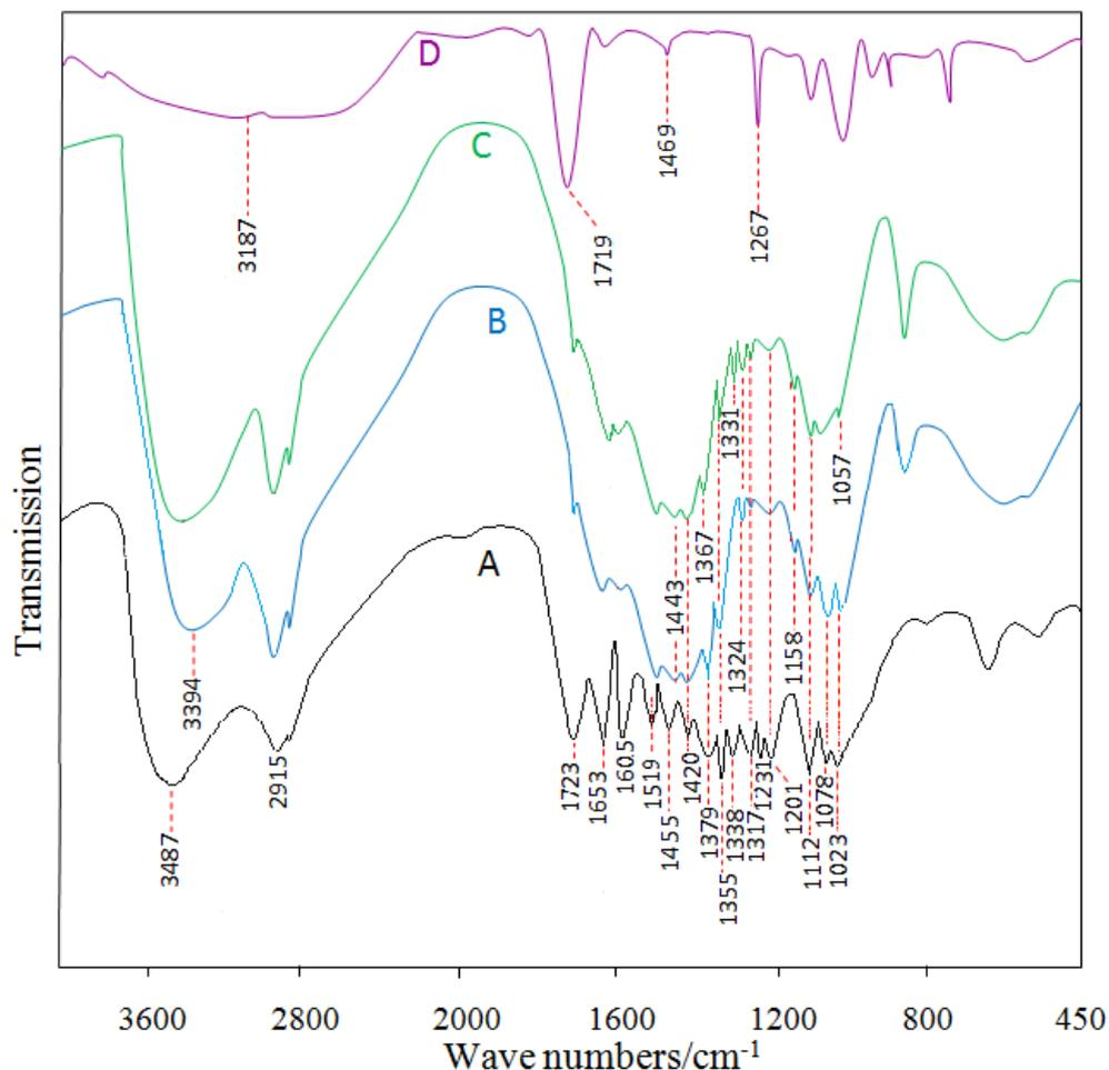
**Figure 3.** FT-IR spectra of LN/PAA hydrogel (A), LN (B), AL (C) and PAA(D)
