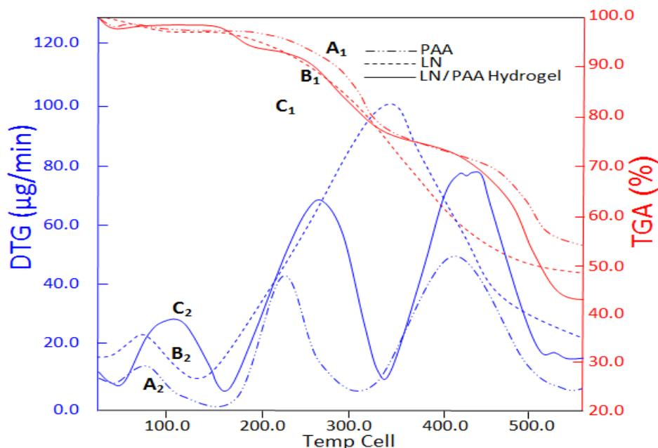
**Figure 4.** TGA and DTG curves in the PAA (A<sub>1</sub> and A<sub>2</sub>), LN (B<sub>1</sub> and B<sub>2</sub>) and LN/PAA hydrogel (C<sub>1</sub> and C<sub>2</sub>)
