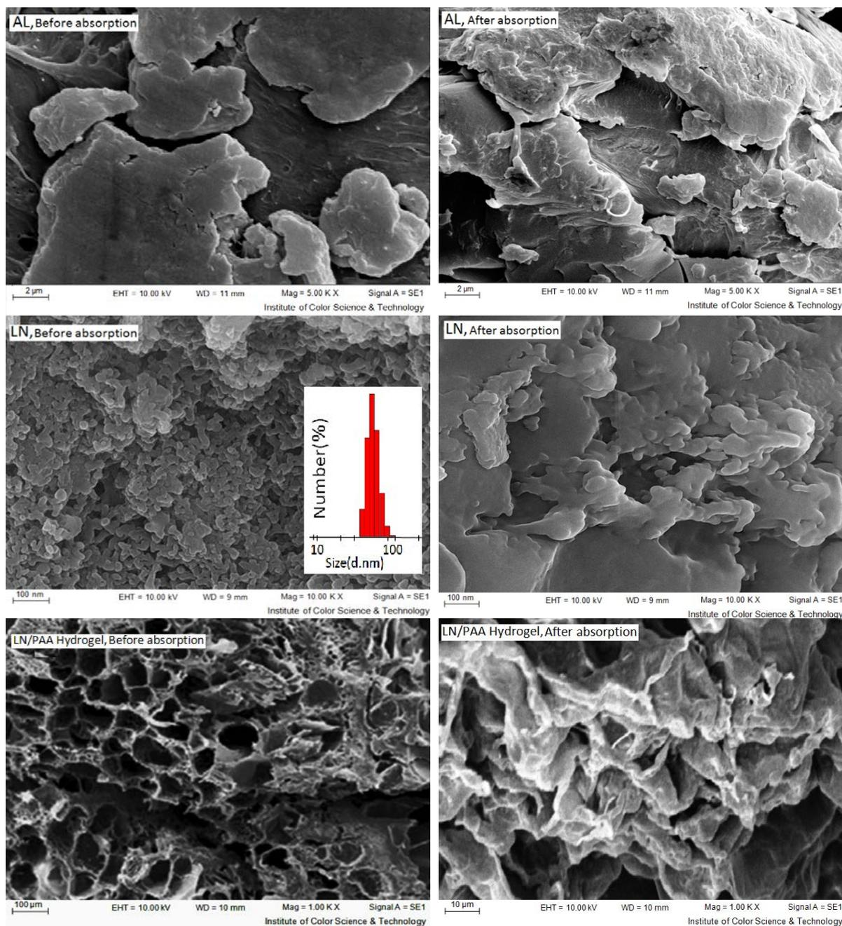
**Figure 2.** SEM images of AL, LN and LN/PAA hydrogel before and after the absorption of Safranin-O dye
