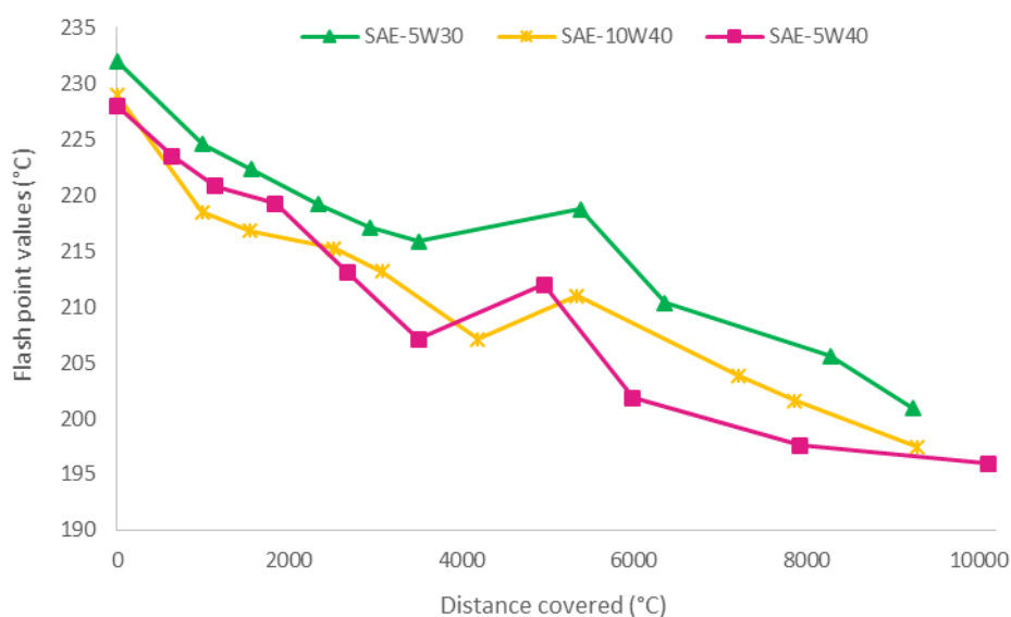
Figure 5. Evolution of the flash point of the lubricating oil versus the distance traveled by the vehicle engine
