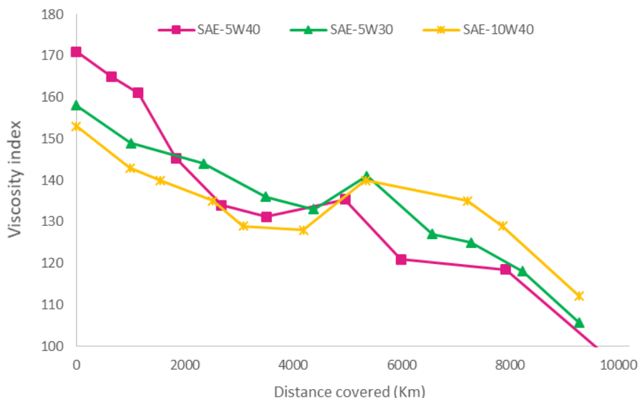
Figure 3. Evolution of the viscosity index of the lubricating oil versus the distance traveled by the vehicle engine
