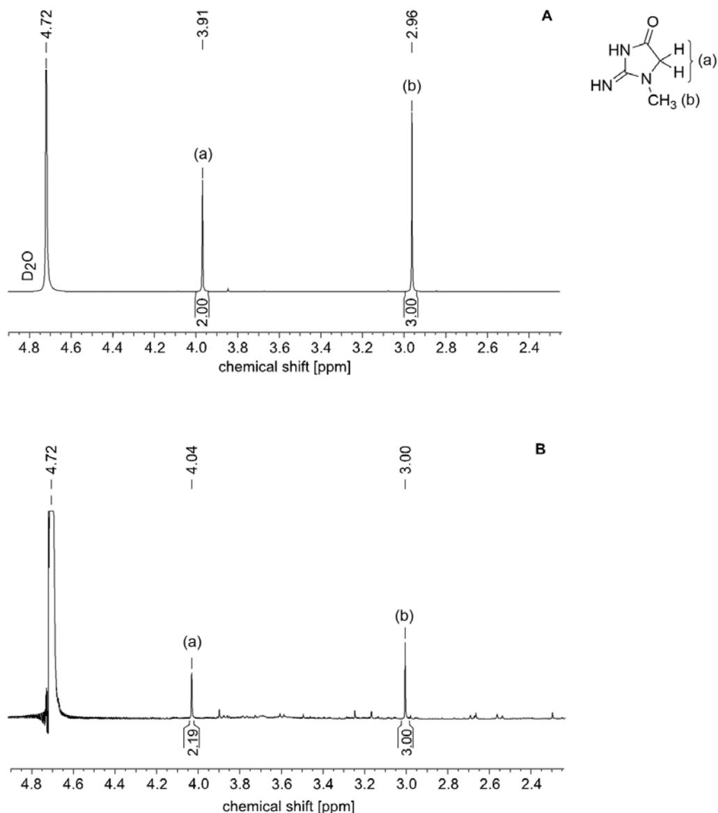
**Figure 1.** A:  $^1\text{H-NMR}$  spectrum of creatinine (1 mg/ml) in deuterium oxide and B:  $^1\text{H-NMR}$  spectrum of a typical urine sample at 600 MHz with water suppression
