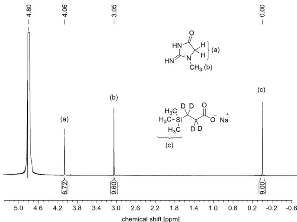
**Figure 2.**  $^1\text{H-NMR}$  spectrum of urine (600 MHz, water suppression) with added standard TSP (0 ppm) for quantification of creatinine concentration. The signals a (4.06 ppm) and b (3.05 ppm) represented the marked protons of creatinine and the signal c (0.00 ppm) represented the marked protons of TSP
