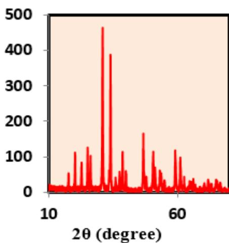
Figure 7. (XRD) diffractogram of CdTiO<sub>3</sub> TF at 400 °C
