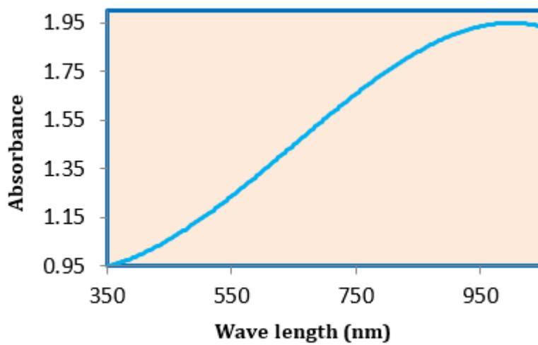
Figure 18. Electronic spectrum of CdTiO<sub>3</sub> TF at 300 °C
