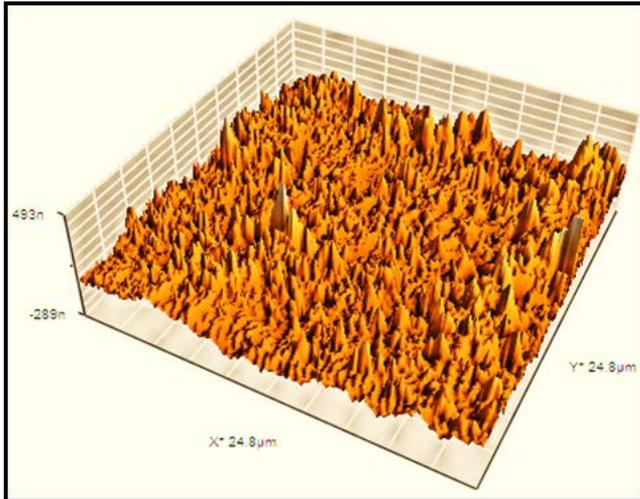
**Figure 12.** (AFM) micrograph of CdTiO<sub>3</sub> TF at 500 °C
