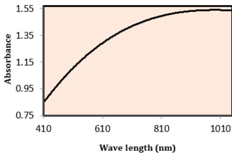
Figure 20. Electronic spectrum of CdTiO<sub>3</sub> TF at 500 °C
