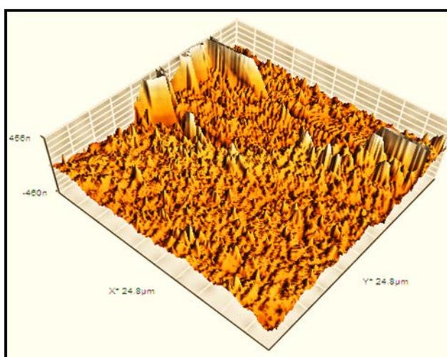
**Figure 11.** (AFM) micrograph of CdTiO<sub>3</sub> TF at 400 °C
