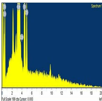
**Figure 3.** (EDS) spectrum of CdTiO<sub>3</sub> TF at 400 °C
