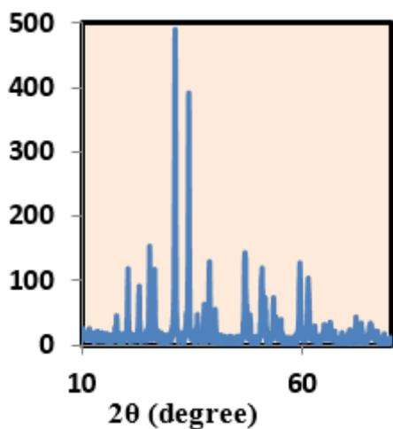
Figure 6. (XRD) diffractogram of CdTiO<sub>3</sub> TF at 300 °C
