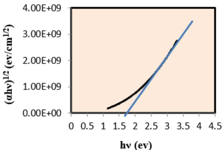
Figure 24. Energy gap of CdTiO<sub>3</sub> TF at 500 °C
