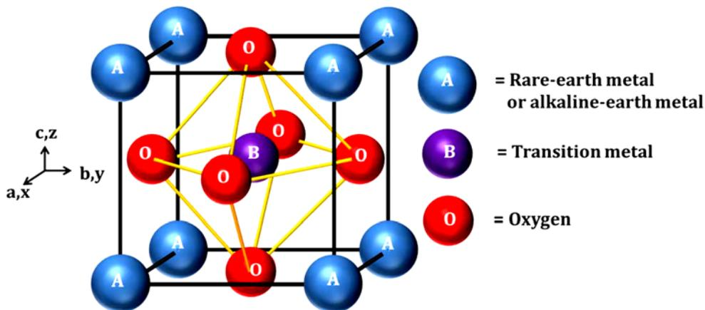
**Figure 1.** Structure of perovskite oxide
