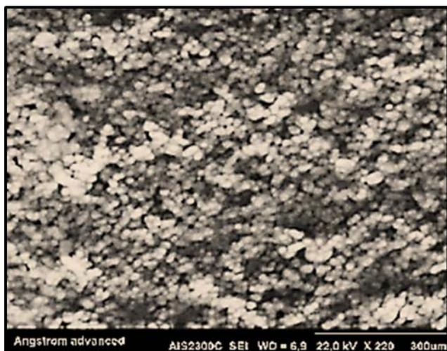
Figure 14. (SEM) image of CdTiO<sub>3</sub> TF at 300 °C
