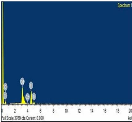
Figure 4. (EDS) spectrum of CdTiO<sub>3</sub> TF at 500 °C
