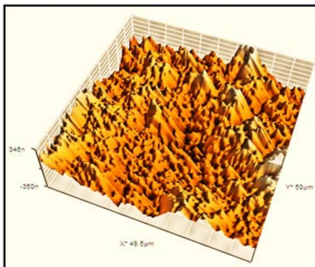
**Figure 10.** (AFM) micrograph of CdTiO<sub>3</sub> TF at 300 °C
