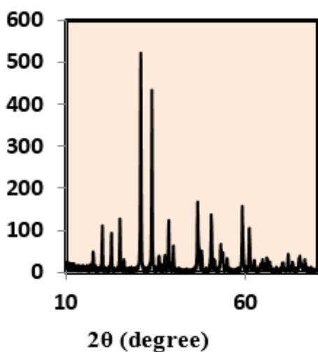
Figure 8. (XRD) diffractogram of CdTiO<sub>3</sub> TF at 500 °C
