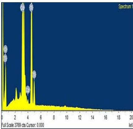
Figure 5. (EDS) spectrum of CdTiO<sub>3</sub> TF at 600 °C
