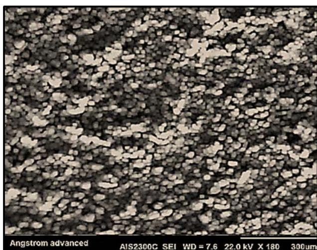
Figure 16. (SEM) image of CdTiO<sub>3</sub> TF at 500 °C
