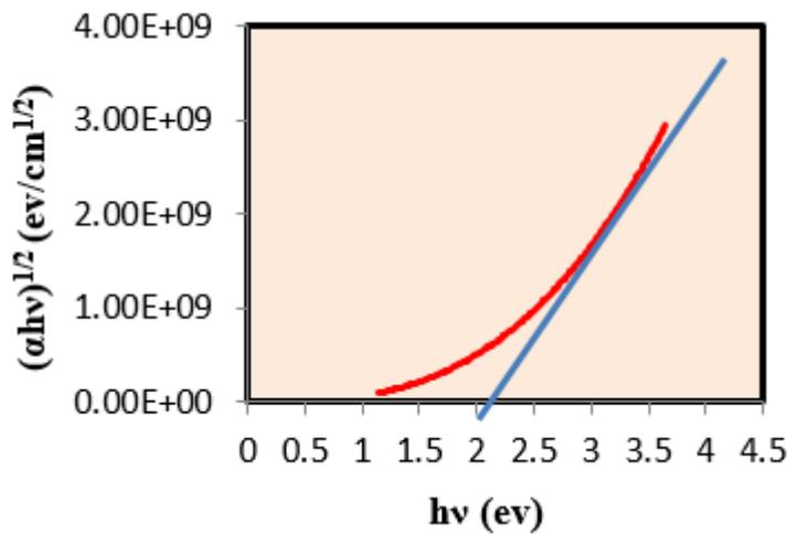
**Figure 23.** Energy gap of CdTiO<sub>3</sub> TF at 400 °C
