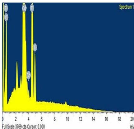
**Figure 2.** (EDS) spectrum of CdTiO<sub>3</sub> TF at 300 °C
