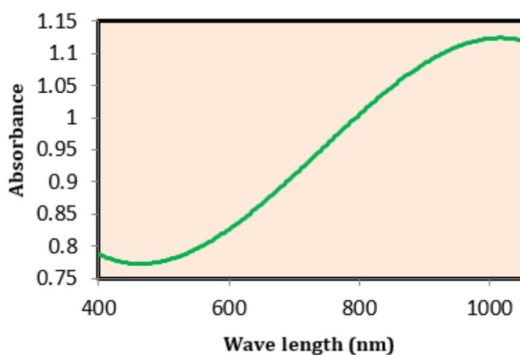
Figure 21. Electronic spectrum of CdTiO<sub>3</sub> TF at 600 °C
