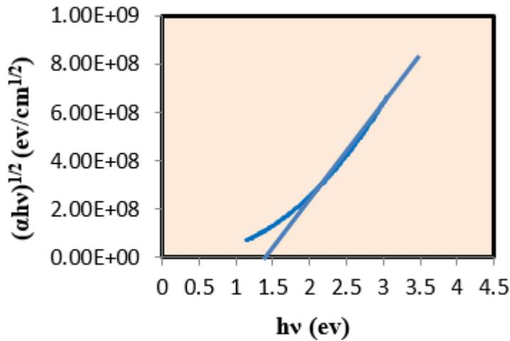
**Figure 22.** Energy gap of CdTiO<sub>3</sub> TF at 300 °C
