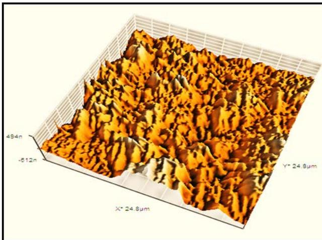
**Figure 13.** (AFM) micrograph of CdTiO<sub>3</sub> TF at 600 °C
