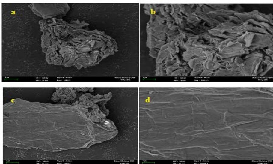
**Figure 4.** FESEM image of GO by oxidation process. Figure (a) and (b) show the porous network of GO, while (c) and (d) show the thin layer of GO
