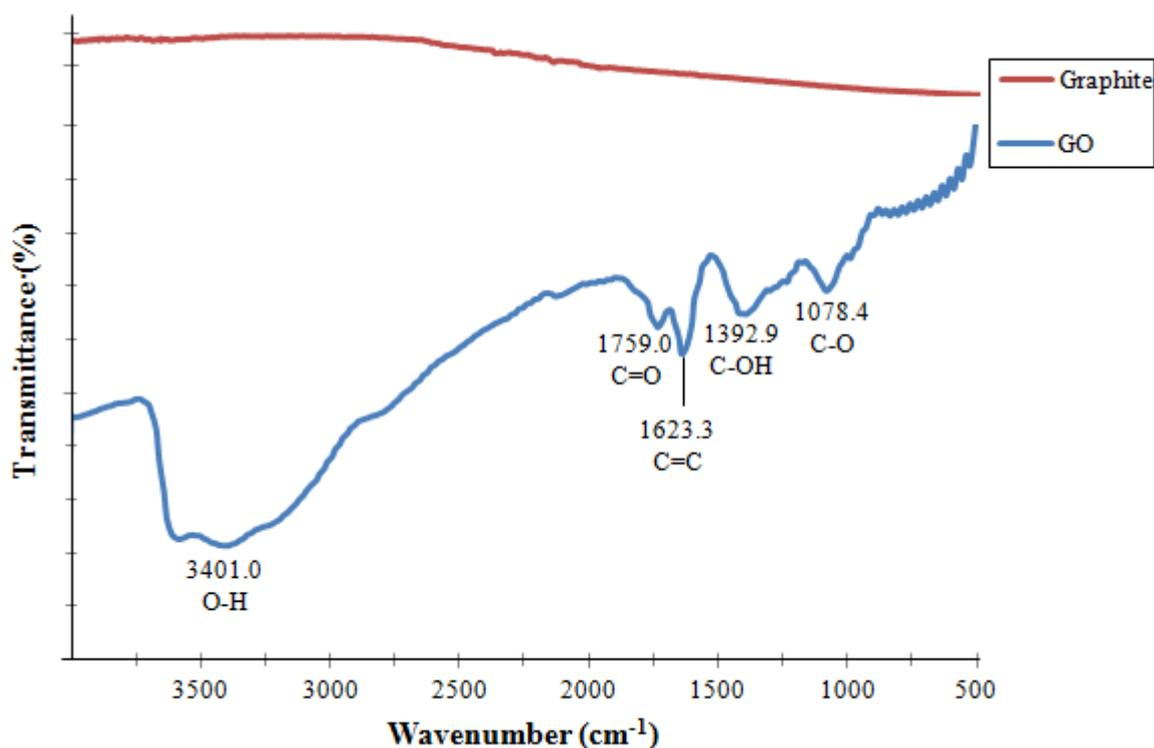
Figure 2. Fourier transform infrared (FT-IR) spectrum of graphene oxide (GO) and graphite
