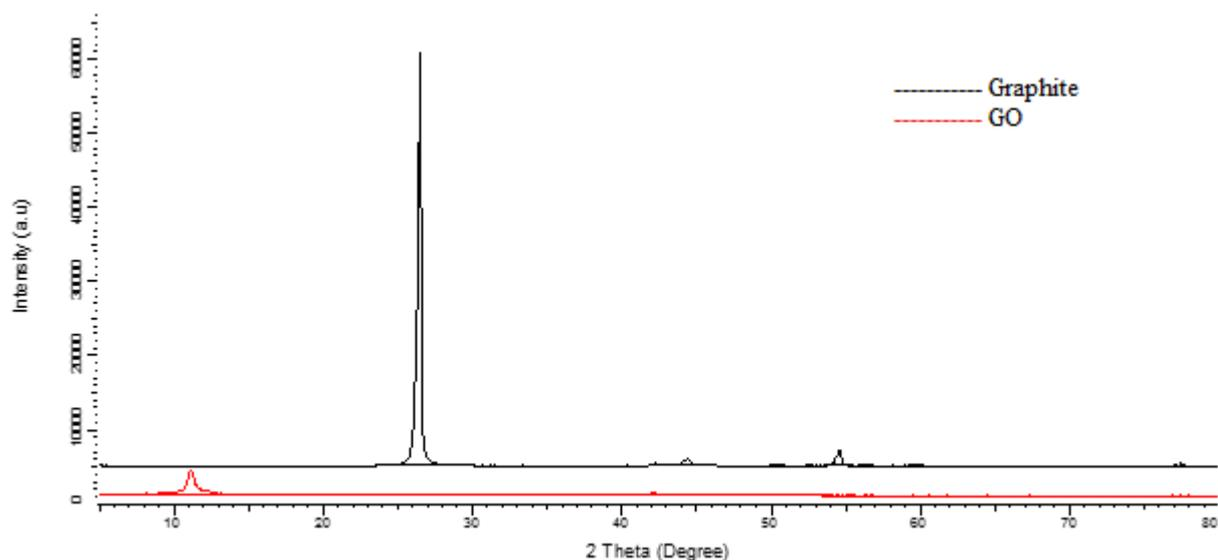
Figure 3. X-ray powder diffraction (XRD) spectrum of graphite and GO
